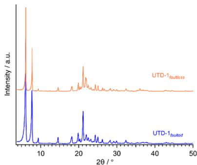
Fig. 1 Powder X-ray diffraction patterns for detemplated UTD-1 (DON) variants.
