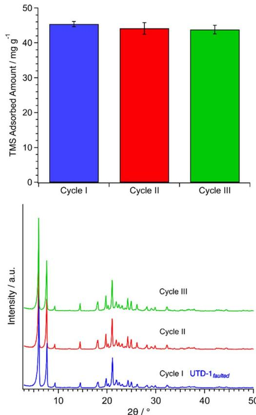
Fig. 7 (Top) Adsorbed amount of TMS onto fresh and regenerated UTD-1<sub>faulted</sub>. (Bottom) XRD pattern of UTD-1<sub>faulted</sub> prior to each adsorption cycle. The initial TMS concentration during the adsorption tests was 125 mg L<sup>-1</sup>. Adsorbent regeneration was performed through thermal treatment and rehydroxylation.
