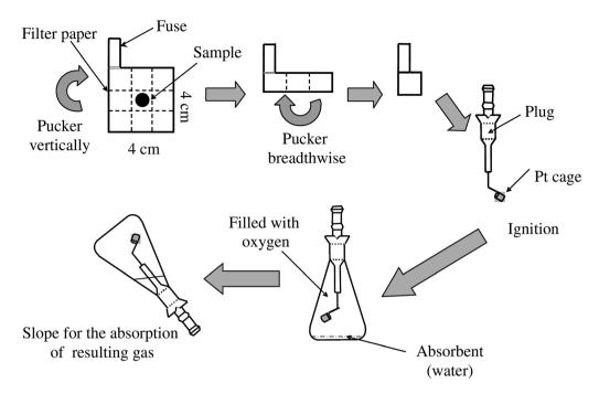
Fig. 2 Procedure of the oxygen flask combustion method.
