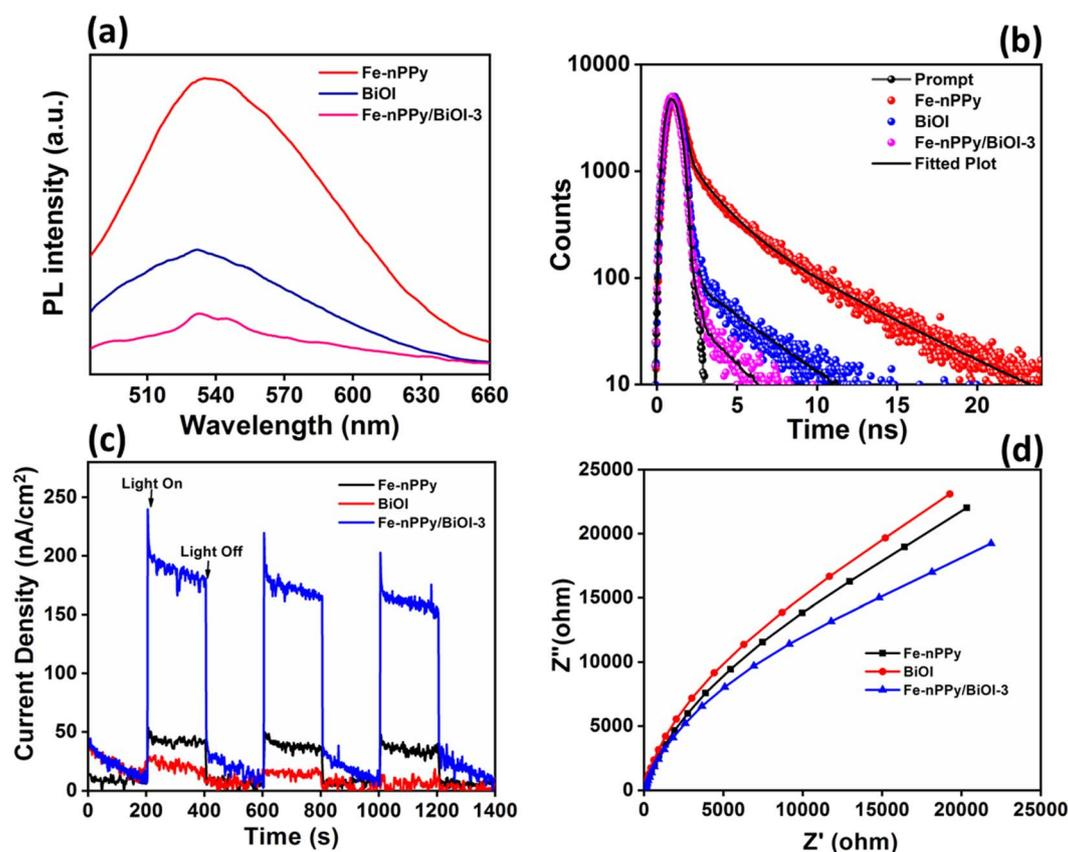
Fig. 10 Photophysical properties of Fe-nPPy, BiOI and Fe-nPPy/BiOI-3 nanocomposite: (a) PL emission spectra, (b) life time decay plots, (c) transient photocurrent responses, and (d) EIS Nyquist plots of nanocomposites.
