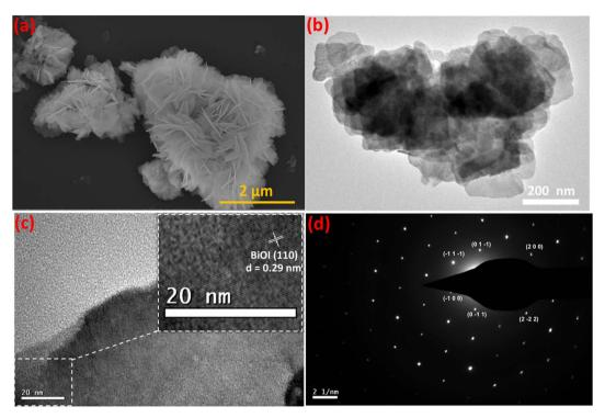
Fig. 5 Particle and microstructure of Fe-nPPy/BiOI-3: (a) FESEM image, (b) TEM image, (c) HRTEM image and (d) SAED pattern.
