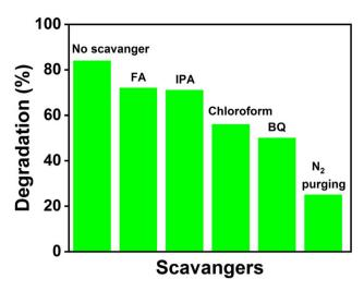
Fig. 11 Scavenger study results of the Fe-nPPy/BiOI-3 photocatalyst for the degradation of CV dye under visible light.
