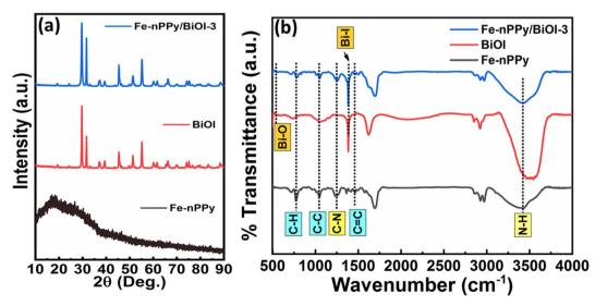
Fig. 2 (a) XRD patterns of Fe-nPPy, BiOI and Fe-nPPy/BiOI-3 and (b) FTIR spectra of Fe-nPPy, BiOI and Fe-nPPy/BiOI-3.
