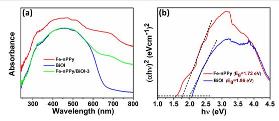
Optical properties of Fe-nPPy, BiOI and Fe-nPPy/BiOI-3: (a) DRS spectra and (b) Tauc plots for band gap calculation of Fe-nPPy and BiOI.
