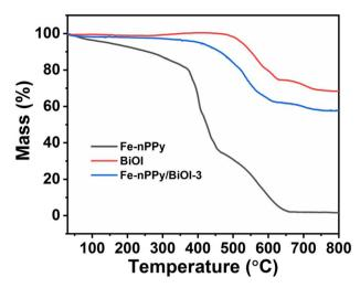
Fig. 3 TGA thermal curves of Fe-nPPy, BiOI and the Fe-nPPy/BiOI-3 nanocomposite under a nitrogen atmosphere.
