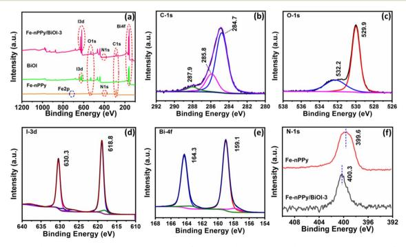
Fig. 4 XPS spectra: (a) survey spectra of Fe-nPPy, BiOI and Fe-nPPy/BiOI-3 and (b) C-1s, (c) O-1s, (d) I-3d and (e) Bi-4f of Fe-nPPy/BiOI-3 and (f) N-1s of Fe-nPPy and Fe-nPPy/BiOI-3.
