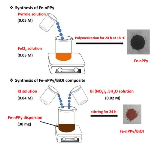
Fig. 1 Schematic representation of the synthesis of Fe-nPPy/BiOI nanocomposites.
