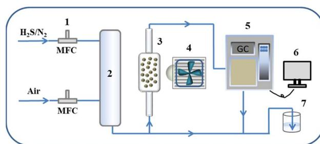
Scheme 1 Schematic diagram of the photocatalytic H<sub>2</sub>S removal process. (1) Mass flow controller; (2) gas mixing tank; (3) reactor; (4) light source; (5) gas chromatograph; (6) computer; (7) tail gas collector.
