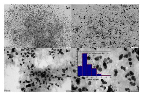
Fig. 2 TEM images at different scales (a; 1 µm, b; 500 nm, (c and d); 100 nm) of AgNPs@chitosan/PVA nanocomposite and average particle size histogram.
