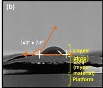
Fig. 10 Contact angle measurement: (a) P. lilacinum,  $147.3 \pm 5.7^{\circ}$  and (b) T. lanuginosus,  $143 \pm 7.6^{\circ}$ .
