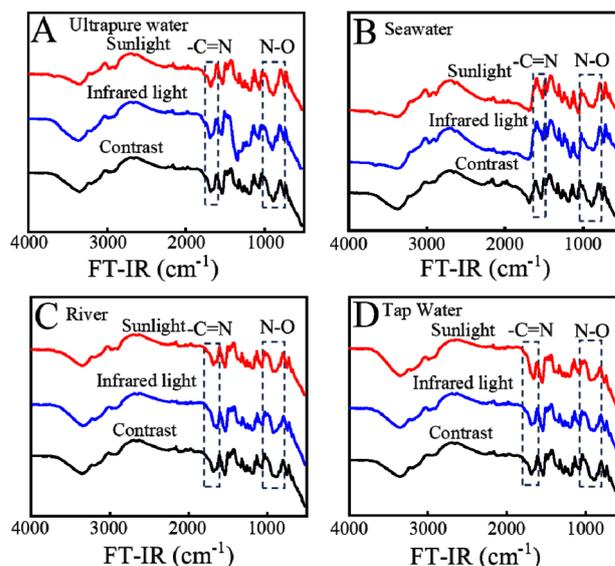
**Fig. 7** FT-IR spectra of U(vi) adsorbed by KMnO<sub>4</sub>@PAO under different illumination and solution conditions.
