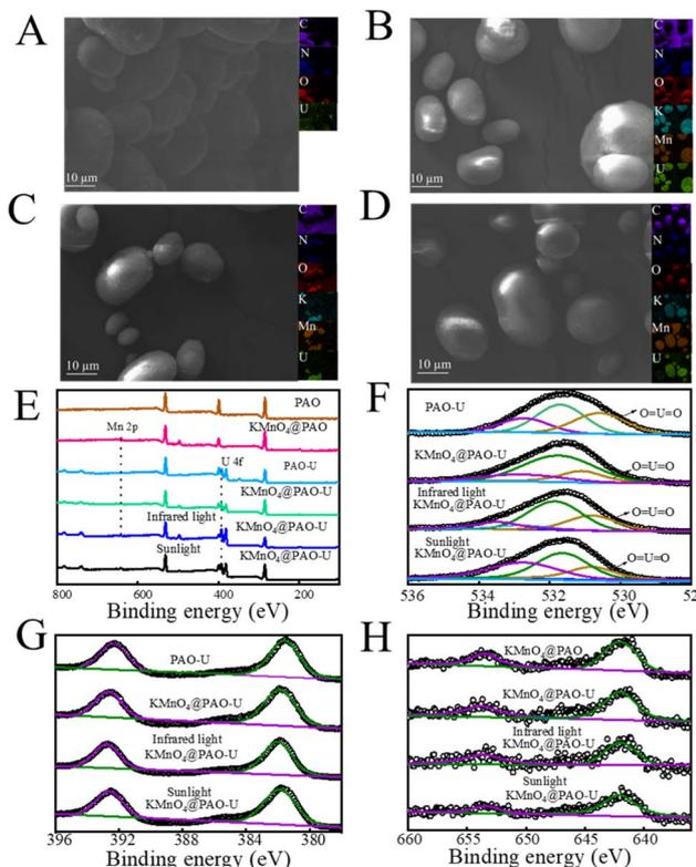
Fig. 8 SEM images of PAO-U (A), KMnO<sub>4</sub>@PAO-U (B), infrared light KMnO<sub>4</sub>@PAO-U (C), and sunlight KMnO<sub>4</sub>@PAO-U (D). XPS survey spectra (E), O 1s (F), U 4f (G), and Mn 2p (H) of PAO-U and KMnO<sub>4</sub>@PAO.
