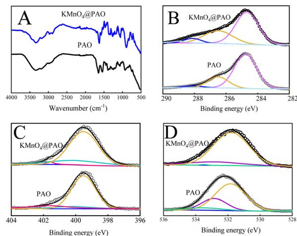
Fig. 3 FT-IR (A), C 1s (B), N 1s (C), and O 1s (D) spectra of  $\text{KMnO}_4\text{@PAO}$  and PAO.
