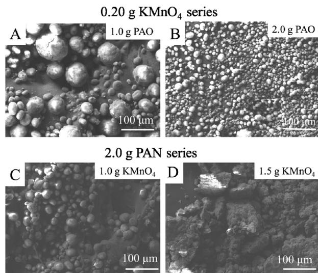
Fig. 2 SEM images of  $\text{KMnO}_4\text{@PAO}$  with different  $\text{KMnO}_4$  and PAO amounts. 0.20 g  $\text{KMnO}_4$  series: 1.0 g PAO (A); 2.0 g PAO (B). 2.0 g PAN series: 1.0 g  $\text{KMnO}_4$  (C); 1.5 g  $\text{KMnO}_4$  (D). The details of  $\text{KMnO}_4\text{@PAO}$  preparation conditions are shown in Table S1.†
