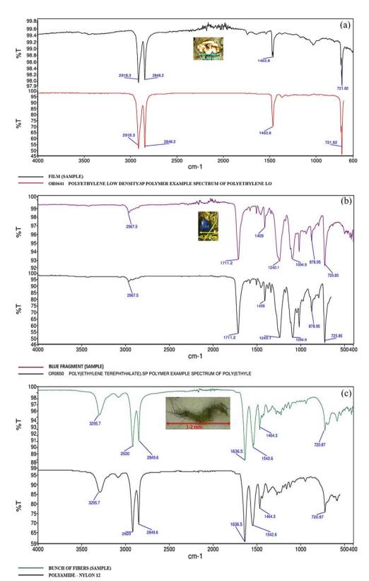
Fig. 5 FTIR spectra of (a) low-density polyethylene (LDPE), (b) polyethylene (PE) and (c) polyamide detected in stormwater samples. The upper line represents the spectra of MP samples in stormwater, and the lower line represents the standard spectra for the reference polymer obtained from the library database.
