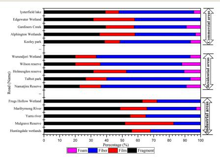
Distribution of total MPs in stormwater based on their shapes, such as fibers, fragments, foams, and films.
