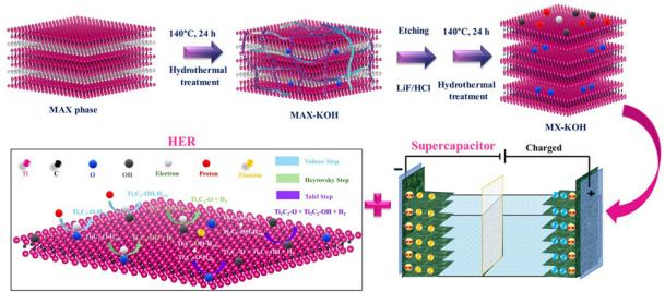
**Supercapacitors with enhanced energy storage and hydrogen evolution reaction performance via sequential alkali-modified MXenes**
