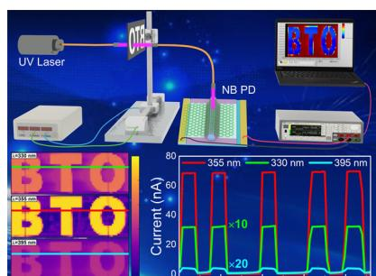
**A power-free, filter-free and high-performance narrowband ZnO/BaTiO<sub>3</sub>/GaN heterojunction-based ultraviolet photodetector obtained by synergetic plasmonic and ferroelectric effects**
