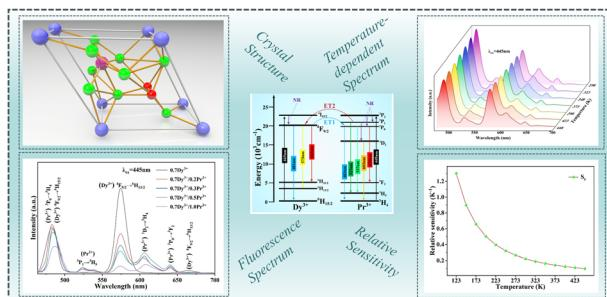
**Highly sensitive temperature sensing of Na(Y<sub>1.5</sub>Na<sub>0.5</sub>)F<sub>6</sub> glass-ceramics based on Dy<sup>3+</sup>/Pr<sup>3+</sup> energy transfer**
