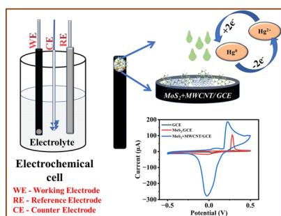
**MoS<sub>2</sub>@MWCNT modified glassy carbon electrode for electrochemical mercury(II) ion sensors**
