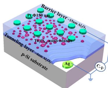
**Atomic layer-deposited  $\text{Ta}_{2}\text{O}_{5-x}$  nano-islands for charge trapping memory devices**
