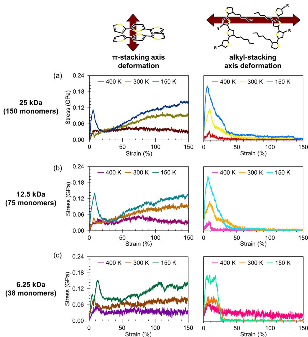
Fig. 6 Simulated stress–strain curves for the crystalline systems along the  $\pi$ -stacking (left) and alkyl-stacking (right) axes; a centered moving average of width 70 ps was applied to the stress values, and the deformation rate was  $5 \times 10^{-4} \text{ nm ps}^{-1}$ . Chain molecular weights of (a) 25 kDa, (b) 12.5 kDa, and (c) 6.25 kDa are explored through independent stress–strain simulations.
