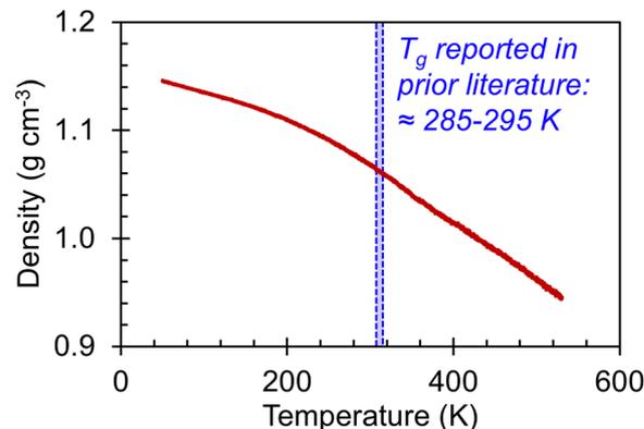
Fig. 2 (red line) Amorphous P3HT system density as a function of temperature during continuous heating from 50 K to 530 K at a rate of  $10 \text{ K ns}^{-1}$ . (blue shaded region) A range of  $T_g$  values previously reported in literature for P3HT.<sup>51–55</sup>
