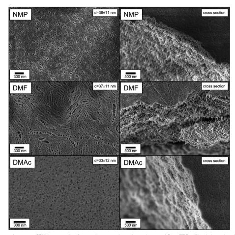
Fig. 3 Scanning electron microscopy (SEM) images of surface and cross sections of membranes of P<sub>27.5</sub> (27.5 wt% cobaltocenium block segment) made of casting solutions of N-methyl-pyrrolidone (NMP) (top), dimethyl formamide (DMF) (middle), and dimethyl acetamide (DMAc) (bottom) with respective pore sizes.
