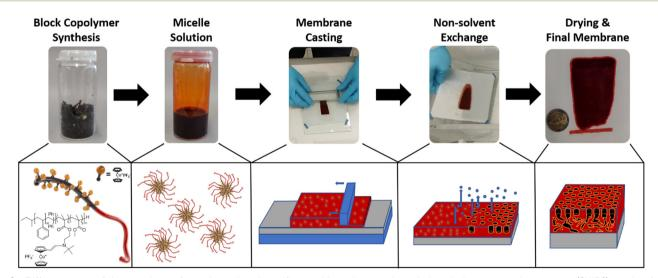
Fig. 2 Different steps of the membrane formation using the self-assembly and non-solvent induced phase separation process (SNIPS) starting from block copolymer (BCP) synthesis, over the formation of a micellar solution, membrane casting, non-solvent exchange and drying to form the final porous membrane.
