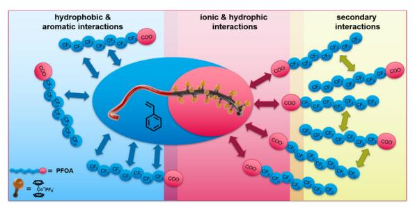
Fig. 1 Possible interaction between the synthesized cobaltocenium-containing block copolymer polystyrene-*b*-(polycobaltoceniumethyl *tert*-butyl aminoethyl methacrylate-*co*-polymethyl methacrylate) (PS-*b*-(PCoEtBAEMA-*co*-PMMA)) and perfluorooctyl acid (PFOA) and resulting secondary interaction effects.
