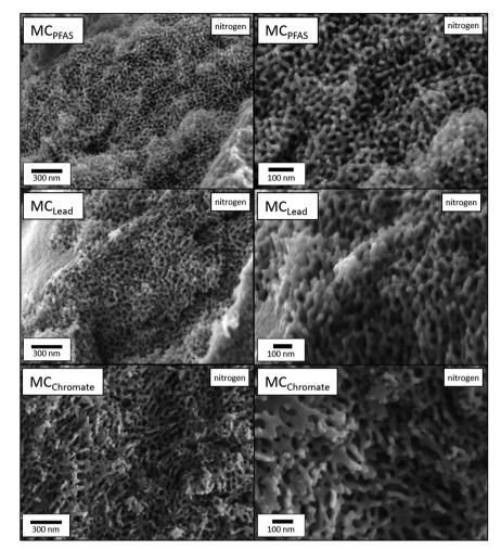
Fig. 6 Scanning electron microscopy (SEM) images of ceramic material formed by template-based calcinating of used membranes in a nitrogen atmosphere to 800 °C. Membrane ceramics after PFOA (MC<sub>PFOA</sub>), lead nitrate (MC<sub>Lead</sub>) and sodium chromate (MC<sub>Chromate</sub>) retention experiments were analysed.
