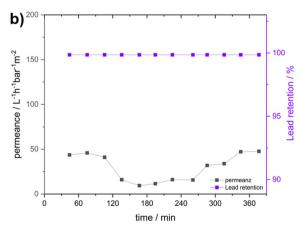
Fig. 5 Water flux combined with sodium chromate and lead nitrate retention measurements analysed inductively coupled plasma mass spectroscopy (ICP-MS); (a) compiled water flux and sodium chromate retention; (b) compiled water flux and lead nitrate retention.
