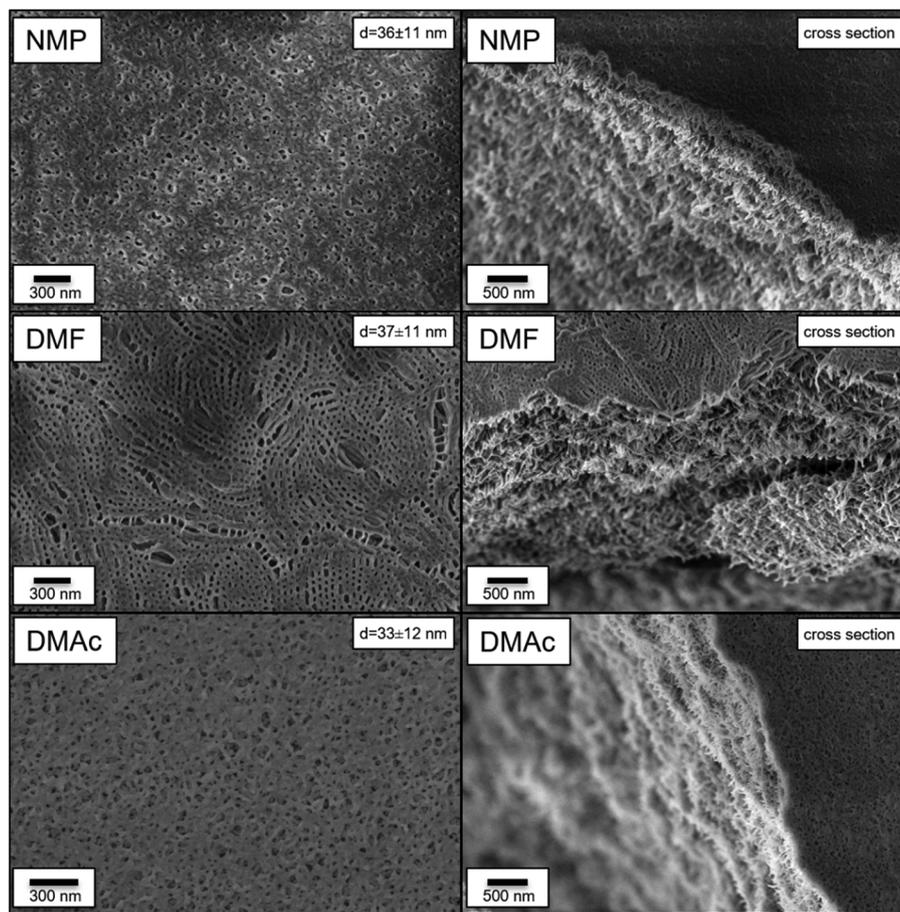
Fig. 3 Scanning electron microscopy (SEM) images of surface and cross sections of membranes of  $P_{27.5}$  (27.5 wt% cobaltocenium block segment) made of casting solutions of *N*-methyl-pyrrolidone (NMP) (top), dimethyl formamide (DMF) (middle), and dimethyl acetamide (DMAc) (bottom) with respective pore sizes.
