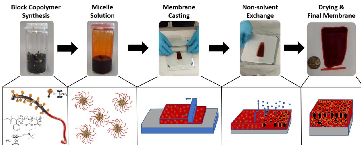
**Fig. 2** Different steps of the membrane formation using the self-assembly and non-solvent induced phase separation process (SNIPS) starting from block copolymer (BCP) synthesis, over the formation of a micellar solution, membrane casting, non-solvent exchange and drying to form the final porous membrane.
