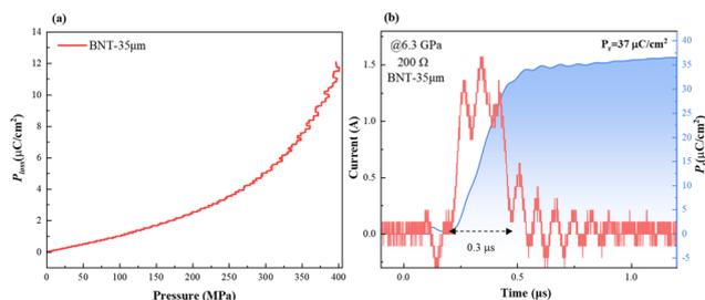
Fig. 8 (a) Depolarization under *in situ* hydrostatic pressure of poled BNT-35  $\mu\text{m}$ ; (b) dynamic response behavior of BNT-35  $\mu\text{m}$  with a 200  $\Omega$  resistor under 6.3 GPa shock pressure.
