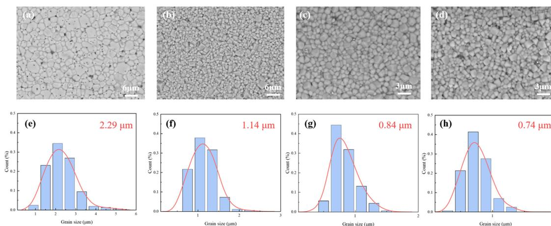
Fig. 3 SEM images and grain size distribution of the BNT–BA–NN MLCCs: (a) and (e) BNT- $88\ \mu\text{m}$ ; (b) and (f) BNT- $78\ \mu\text{m}$ ; (c) and (g) BNT- $35\ \mu\text{m}$ ; (d) and (h) BNT- $28\ \mu\text{m}$ .
