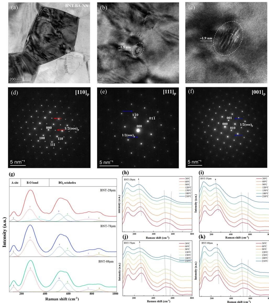
Fig. 5 (a)–(c) Bright-field TEM micrographs and (d)–(f) selected-area electron diffractions (SAED) patterns of BNT-28  $\mu\text{m}$  MLCC; (g) Raman spectra of BNT MLCCs at room temperature; (h)–(k) temperature-dependent Raman spectra of BNT MLCCs.
