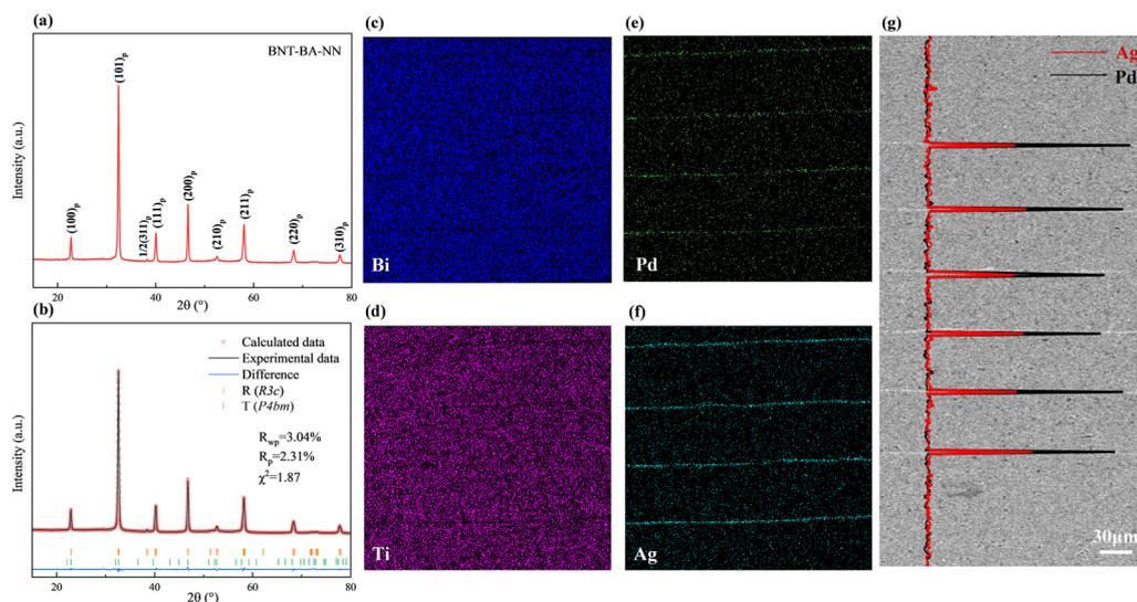
Fig. 2 (a) XRD pattern and (b) Rietveld refinement of BNT-BA-NN ceramic powder from  $25^\circ$  to  $80^\circ$ , (c)–(f) the EDS images of the Bi, Ti, Pd and Ag elements; (g) the EDS line scanning result of Ag/Pd elements in the multilayer structure.
