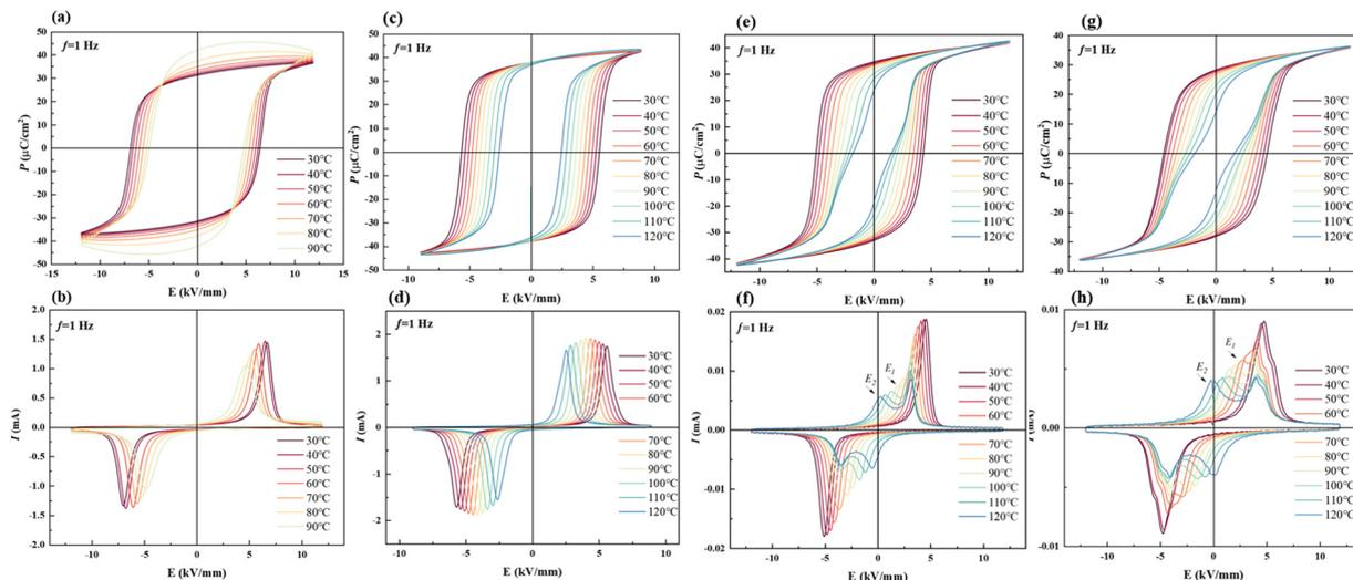
Fig. 6 Temperature-dependent (a)  $P$ - $E$  loops and (b)  $I$ - $E$  curves of the BNT-88  $\mu\text{m}$  MLCC at  $12 \text{ kV mm}^{-1}$ ; (c)  $P$ - $E$  loops and (d)  $I$ - $E$  curves of the BNT-78  $\mu\text{m}$  MLCC at  $9 \text{ kV mm}^{-1}$ ; (e)  $P$ - $E$  loops and (f)  $I$ - $E$  curves of the BNT-35  $\mu\text{m}$  MLCC at  $12 \text{ kV mm}^{-1}$ ; (g)  $P$ - $E$  loops and (h)  $I$ - $E$  curves of the BNT-28  $\mu\text{m}$  MLCC at  $12 \text{ kV mm}^{-1}$ .
