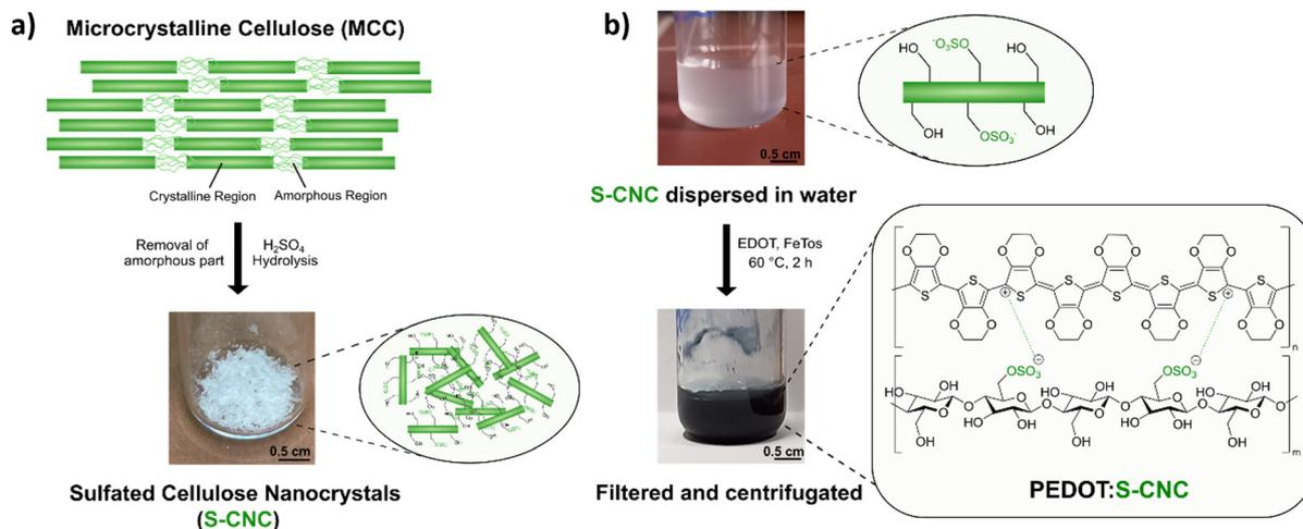
**Fig. 1** (a) Illustration of deconstruction from microcrystalline cellulose (MCC) *via* sulfuric acid ( $\text{H}_2\text{SO}_4$ ) hydrolysis to the produced sulfated cellulose nanocrystals (S-CNCs). (b) The S-CNCs dispersed in water (semi-transparent) changes color to a dark blue upon oxidative chemical polymerization with EDOT and FeTos. The shown molecular structures are linked to the photos of the colloidal solutions.
