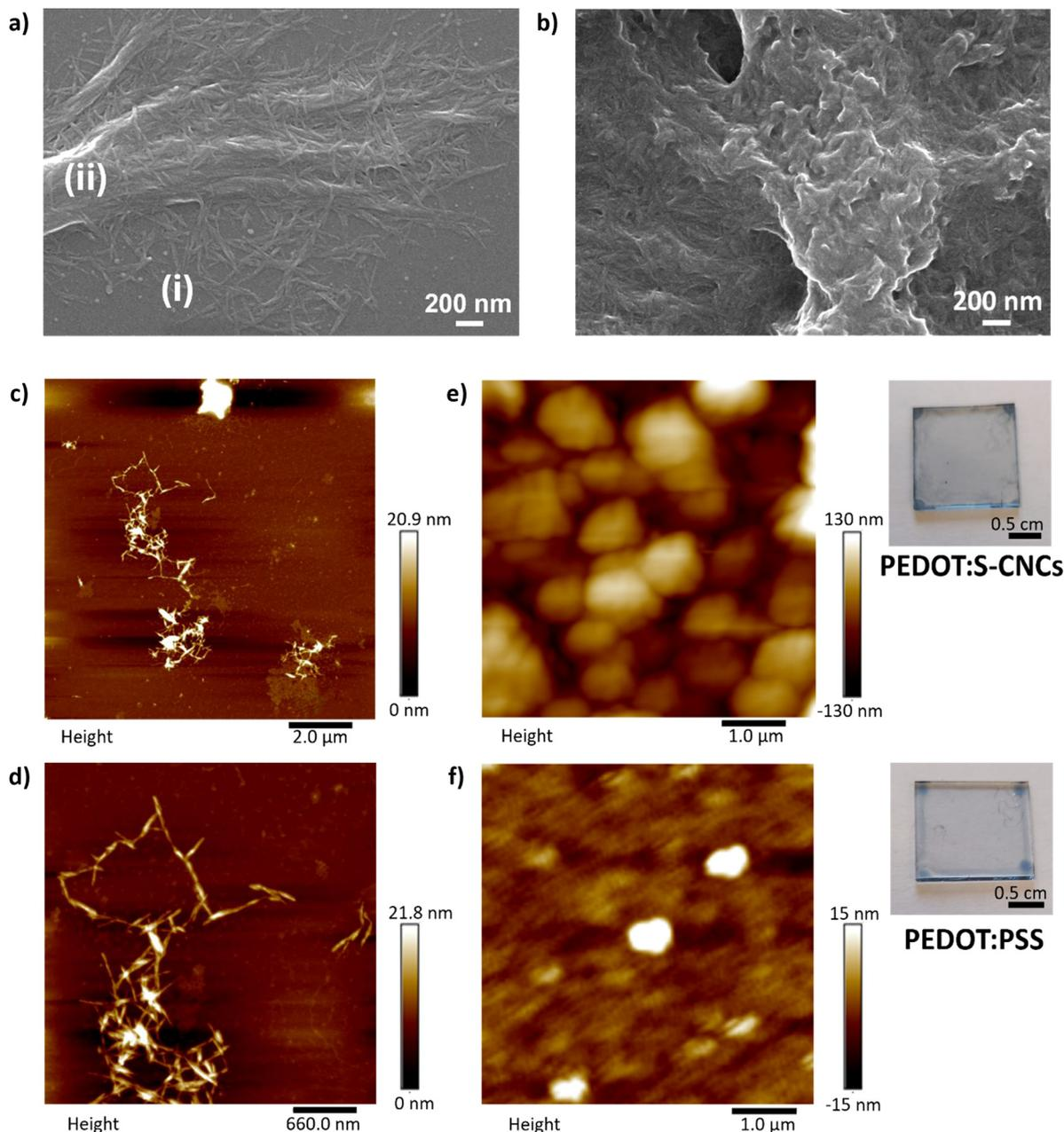
**Fig. 3** FE-SEM micrographs (120 000 $\times$ ) (a) of the pristine S-CNCs<sup>30</sup> and (b) the PEDOT:S-CNCs composite. Scale bar 200 nm. Atomic force microscopy (AFM) images of (c) and (d) pristine S-CNCs and (e) the PEDOT:S-CNCs composite (thickness = 250 nm), and (f) PEDOT:PSS (thickness = 260 nm). The photographs of composites thin-films on the right side of the respective AFM images.
