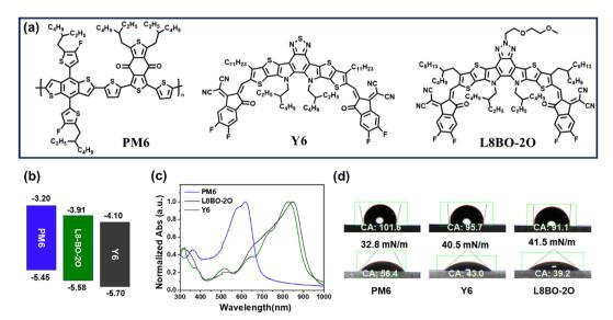
Fig. 1 (a) Chemical structures of donor PM6 and two acceptors Y6, L8BO-2O. (b) Energy levels of PM6, Y6 and L8BO-2O. (c) UV-vis spectra of PM6, Y6 and L8BO-2O neat films. (d) The contact angles of water (top panel) and diiodomethane (bottom panel) droplets on PM6, Y6 and L8BO-2O neat films.
