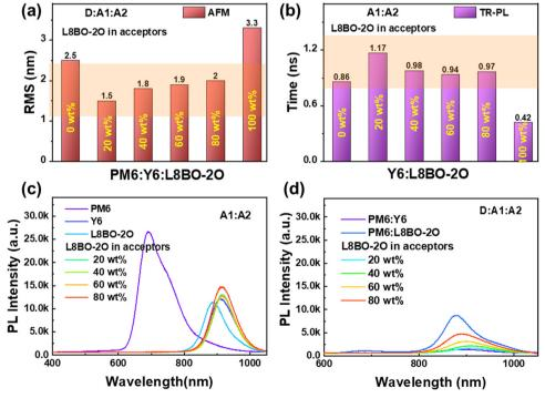
Fig. 2 (a) RMS surface roughness values of the PM6:Y6:L8BO-2O blend films with different L8BO-2O contents. (b) Exciton lifetimes of Y6, L8BO-2O and mixed acceptor films. (c) PL spectra of PM6, Y6, L8BO-2O neat films and mixed acceptor films. (d) PL spectra of binary and ternary blend films.
