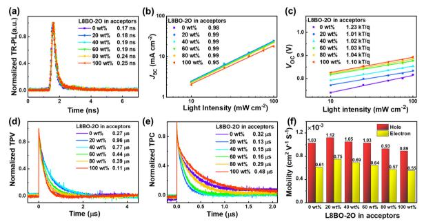
Fig. 4 (a) TR-PL curves of binary and ternary blend films. (b) J<sub>SC</sub>s and (c) V<sub>OC</sub>s versus light illumination intensity of the corresponding OSCs. (d) TPV and (e) TPC curves of the corresponding OSCs. (f) Hole and electron mobilities of the binary and ternary blend films.
