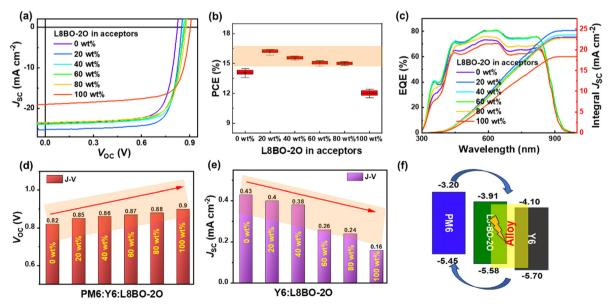
Fig. 3 (a) J-V curves, (b) device efficiency statistics obtained from ten devices, (c) the corresponding EQE spectra and (d)  $V_{OC}$ s of PM6:Y6:L8BO-2Obased OSCs with different L8BO-2O contents. (e) The J-V curves of Y6, L8BO-2O and Y6:L8BO-2O-based pure acceptor devices. (f) Schematic diagram of the working mechanism
