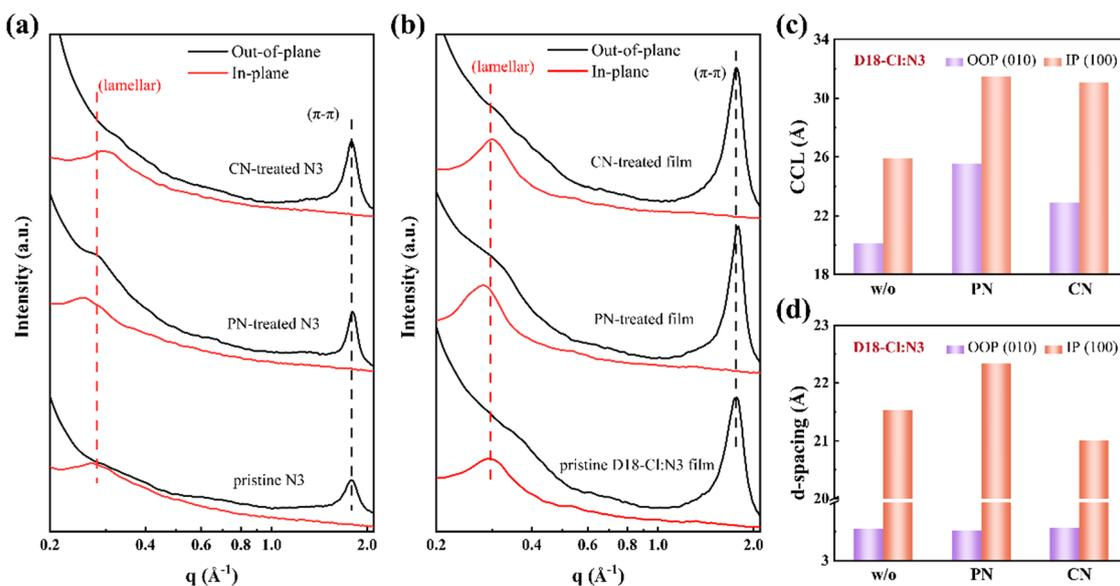
Fig. 2 (a) and (b) The GIXRD profiles of neat N3 and D18-Cl:N3 blend films without and with different additives (0.5 vol%). (c) The calculated CCLs and (d)  $d$ -spacing variation in the D18-Cl:N3 blend films without and with different additives (0.5 vol%).
