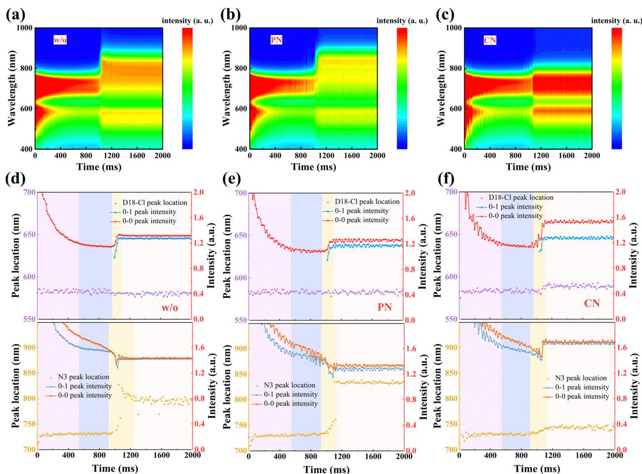
Fig. 3 Time-dependent contour maps of *in situ* UV-Vis absorption spectra of the D18-Cl:N3 samples processed (a) without any additives (b) with 0.5 vol% PN and (c) with 0.5 vol% CN. Time evolution of the peak location and intensity of the donor and acceptor in the D18-Cl:N3 samples processed (d) without any additives (e) with 0.5 vol% PN and (f) with 0.5 vol% CN.
