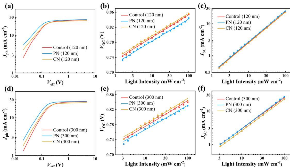
Fig. 5 (a)–(c)  $J_{ph}$ – $V_{eff}$  curves and the dependence of  $V_{OC}$  and  $J_{SC}$  on the light intensity of the 120-nm-thick D18-Cl:N3 OSCs. (d)–(f)  $J_{ph}$ – $V_{eff}$  curves and the dependence of  $V_{OC}$  and  $J_{SC}$  on the light intensity of the 300 nm-thick D18-Cl:N3 OSCs.
