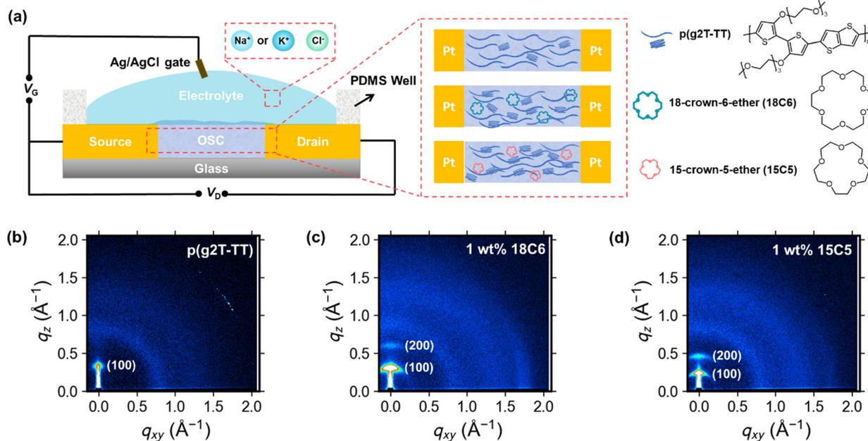
Fig. 1 (a) The schematic representation of organic electrochemical transistor (OECT) in this study with different active materials membrane: pristine p(g2T-TT); 18C6-mixed p(g2T-TT) and 15C5-mixed p(g2T-TT). The electrolyte in OECT was 0.1 M NaCl or KCl aqueous solution. Comparison of grazing incidence wide-angle X-ray scattering (GIWAXS) 2D patterns of polymer thin films after annealing at 125 °C for 10 minutes: (b) p(g2T-TT), (c) 1 wt% 18C6-mixed p(g2T-TT) and (d) 1 wt% 15C5-mixed p(g2T-TT).
