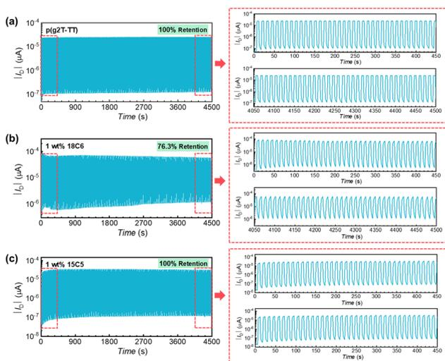
Fig. 5 Operational stability of drain current for OECTs. Transient responses of the drain current for  $V_D$  is  $-0.4$  V and square pulse  $V_G$  switching between 0 and  $-0.4$  V with the pulse width of 5 s for 450 cycles in 0.1 M NaCl aqueous solution. The right figures show the first 45 cycles (top) and the last 45 cycles (bottom): (a) pristine p(g2T-TT); (b) 18C6-mixed p(g2T-TT), and (c) 15C5-mixed p(g2T-TT).
