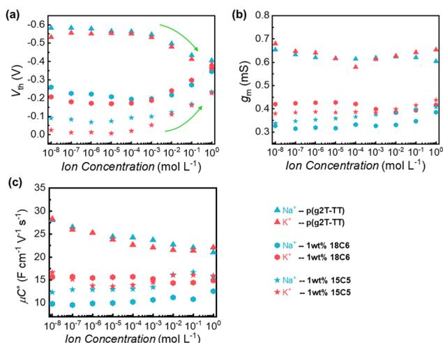
Fig. 3 Concentration dependence for (a)  $V_{th}$ , (b)  $g_m$ , and (c)  $\mu C^*$  in transfer characteristics. The results of p(g2T-TT) stand as triangle markers, hexagon as 1 wt% 18C6-mixed p(g2T-TT), and star as 1 wt% 15C5-mixed p(g2T-TT). Blue markers show the data obtained by using the NaCl aqueous solution as the electrolyte and the red ones by using the KCl aqueous solution.
