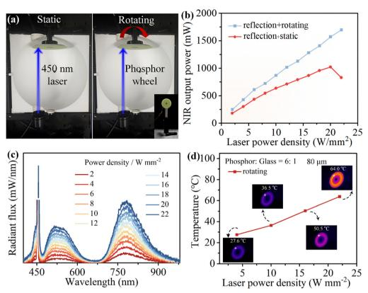
Fig. 5 (a) Digital photograph of the self-built laser system using a reflective light path and the fabricated phosphor wheel installed inside an integrating sphere. (b)  $P_{\rm in}$ -dependent NIR output power of the optimal CSSO:Ce,Cr,Li PiGF-on-sapphire sample in static and rotating excitation modes. (c) EL spectra of the phosphor wheel when rotating under blue laser irradiation at different  $P_{in}$  values. (d) The  $P_{in}$ -dependent real-time temperature at the laser spot when rotating
