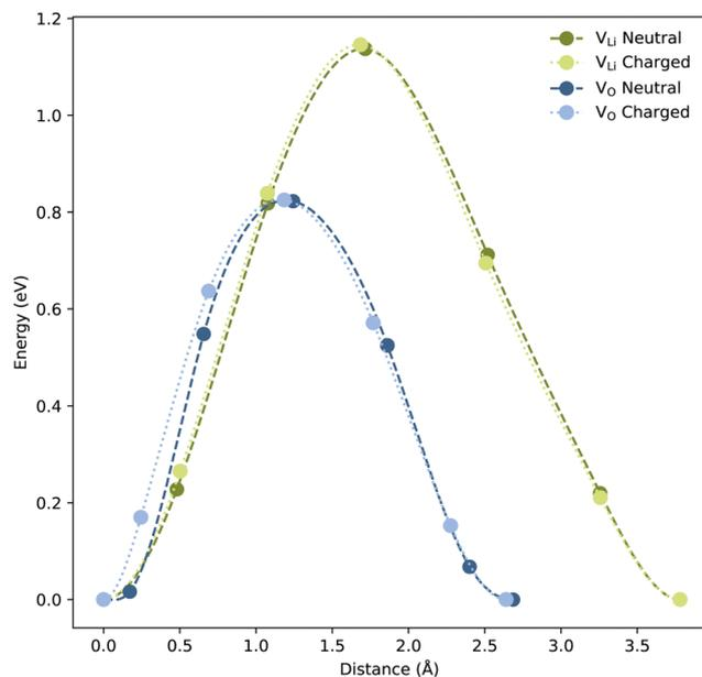
Fig. 4 Migration barriers for both neutral and charged  $V_{Li}$  and  $V_O$  in the  $LiNbO_3$  bulk structure. Energy, normalised to the initial structure, is plotted as a function of the distance moved by the defect. The charge of the charged cells including  $V_{Li}$  and  $V_O$  are  $-1$  and  $+2$ , respectively.
