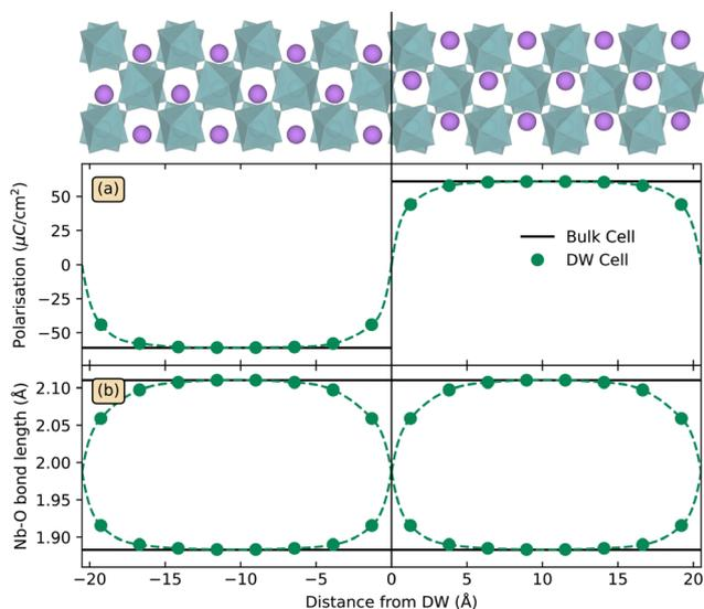
**Fig. 1** Structural parameters for a 160 atom Y-type DW cell as a function of distance from the domain wall. Panel (a) displays polarisation calculated using the point charge model, and panel (b) shows Nb–O bond lengths. The domain wall cell is displayed at the top with the DW marked by the solid black line, with oxygen atoms omitted for clarity.
