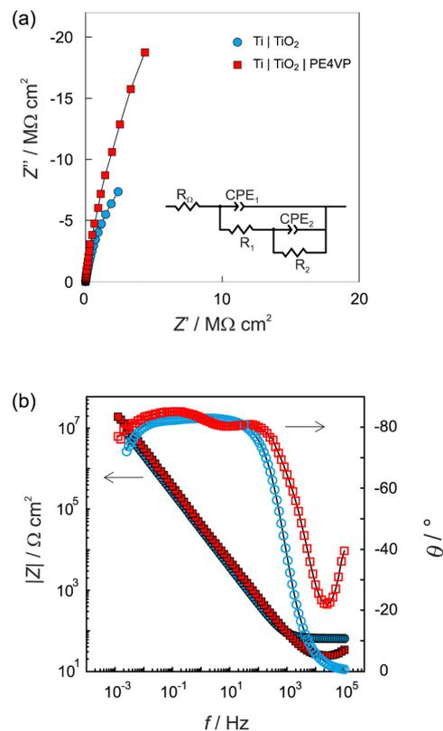
Fig. 10 The Nyquist (a) and Bode (b) plots of the modified Ti electrodes, Ti|TiO<sub>2</sub> (●) and Ti|TiO<sub>2</sub>|PE4VP (■) recorded at EOC in 0.1 mol dm<sup>-3</sup> sodium chloride after 1 hour stabilization. The inset shows the EEC used for EIS data modelling. The experimental data are represented by the symbols, while the solid lines indicate data obtained from EEC modelling.
