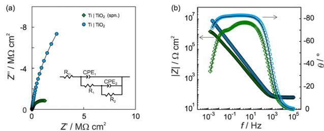
Fig. 5 The Nyquist (a) and Bode (b) plots of the unmodified ( $\text{Ti}|\text{TiO}_2(\text{spn})$ :  $\blacklozenge$ ) and modified ( $\text{Ti}|\text{TiO}_2$ :  $\bullet$ ) electrodes recorded at  $E_{\text{OC}}$  in  $0.1 \text{ mol dm}^{-3}$  sodium chloride after 1 hour stabilization. Inset: The EEC used for EIS data modelling. The experimental data are represented by the symbols, while the solid lines indicate data obtained from EEC modelling.
