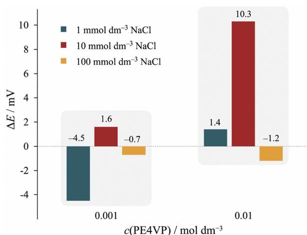
Fig. 9 The difference in the measured open circuit potential of uncoated Ti|TiO<sub>2</sub> and PE4VP coated Ti|TiO<sub>2</sub>|PE4VP electrode for different concentrations of sodium chloride and PE4VP at 25 °C.
