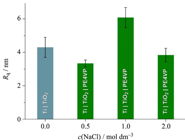
Fig. 7 Surface roughness of the unmodified Ti|TiO<sub>2</sub> sample and Ti|TiO<sub>2</sub> sample coated with PE4VP in the presence of different NaCl concentrations.
