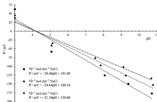
Fig. 3 Inner surface potential of the Ti|TiO<sub>2</sub> sample evaluated from the OCP signal at 25 °C in sodium chloride aqueous solution of concentration: (●)  $10^{-3}$  mol dm<sup>-3</sup>; (▲)  $10^{-2}$  mol dm<sup>-3</sup>; (◆)  $10^{-1}$  mol dm<sup>-3</sup>.
