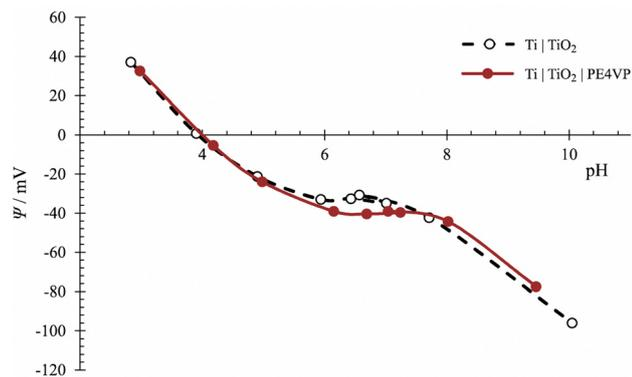
Fig. 8 Inner surface potential of the uncoated Ti|TiO<sub>2</sub> (○) and PE4VP (●) coated Ti|TiO<sub>2</sub>|PE4VP electrode in 0.1 mol dm<sup>-3</sup> aqueous sodium chloride solution at 25 °C. The concentration of PE4VP aqueous solution used for coating of the Ti|TiO<sub>2</sub> surface was 0.01 mol dm<sup>-3</sup>.
