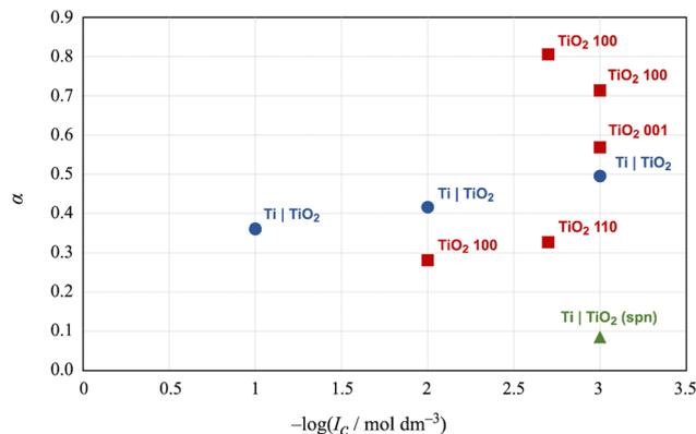
Fig. 4 Comparison of the  $\alpha$  parameter for different  $\text{TiO}_2$  surfaces obtained by means of  $\text{TiO}_2$  electrodes and the OCP method: ( $\blacktriangle$ )  $\text{Ti}|\text{TiO}_2(\text{spn})$ ; ( $\bullet$ )  $\text{Ti}|\text{TiO}_2$  and ( $\blacksquare$ ) rutile (100), (001), and (110) planes.<sup>28</sup>
