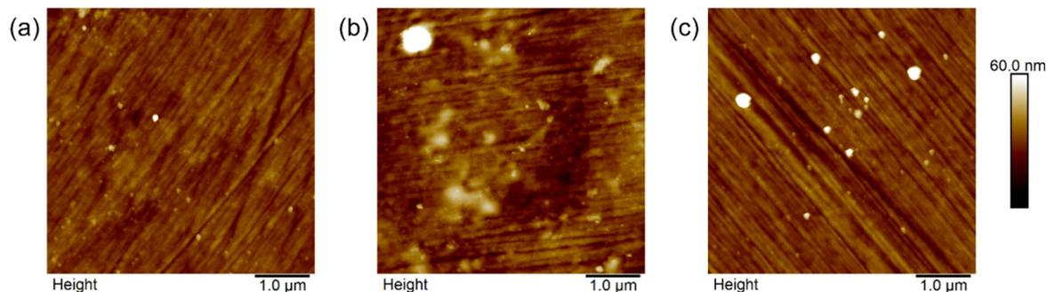
Fig. 6 AFM images of the electrochemically modified Ti|TiO<sub>2</sub> surface after adsorption of PE4VP on it in the presence of (a) 0.5 mol dm<sup>-3</sup>, (b) 1.0 mol dm<sup>-3</sup>, and (c) 2.0 mol dm<sup>-3</sup> NaCl.
