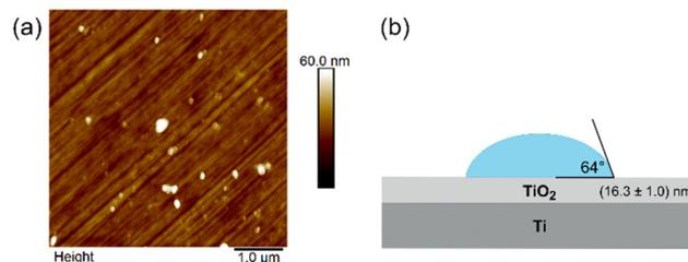
Fig. 2 Surface characterisation of the Ti|TiO<sub>2</sub> sample: (a) AFM image and (b) results of contact angle and ellipsometry measurements.
