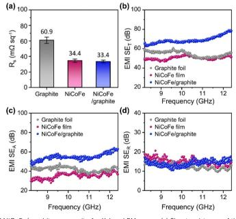
Fig. 3 EMI shielding performance of NiCoFe/graphite composite for X-band EM waves. (a) Sheet resistance of the graphite foil, NiCoFe alloy film, and NiCoFe/graphite composite. (b)-(d) EMI shielding effectiveness of the graphite foil, NiCoFe alloy film, and NiCoFe/graphite composite: (b) total shielding effectiveness, (c) absorption loss, and (d) reflection loss
