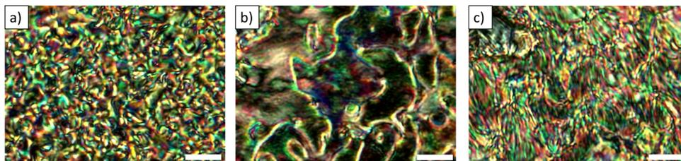
Fig. 3 Optical textures of **CBCOO5CB** obtained on cooling. (a) The schlieren texture of the N phase at 56 °C. (b) The blocky texture of the  $N_{TB}$  at 41 °C. (c) The rope texture of the  $N_{TB}$  phase at 28 °C. The scale bar is 10  $\mu\text{m}$ .
