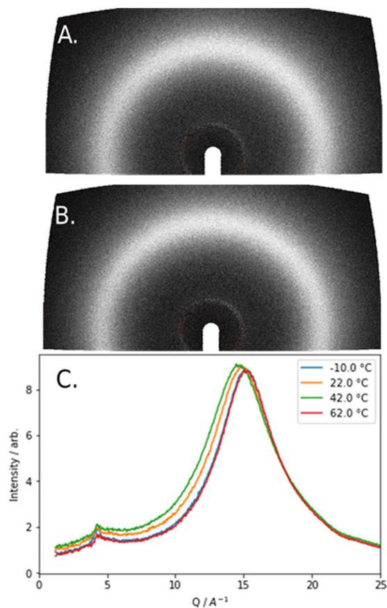
Fig. 4 2D SAXS patterns for (A) **CBCOO7CB** in the nematic phase at 50 °C; (B) **CBCOO7CB** in the  $N_{TB}$  phase at 30 °C. (C) plot of integrated scattering intensity versus  $Q$  at a range of temperatures.
