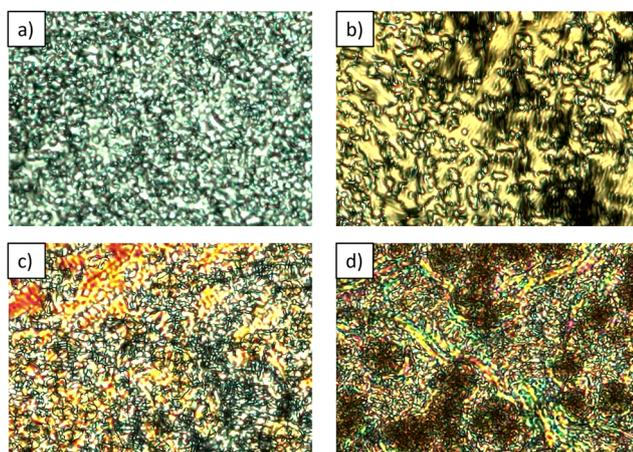
Fig. 7 Optical textures of **CBCONH5CB** obtained on cooling. (a) The thread-like texture of the  $N$  phase at 79 °C. (b) The blocky texture of the  $N_{\text{TB}}$  at 71 °C. (c) Texture of the  $N_{\text{TB}}$  phase at 71 °C upon standing. (d) Texture of the  $N_{\text{TB}}$  phase and crystallization occurring at 58 °C. The scale bar is 10  $\mu\text{m}$ .
