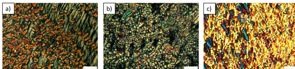
Fig. 6 Optical textures of **S-CBCOO7CB** in the  $N_{\text{TB}}$  phase obtained on cooling in a 5  $\mu\text{m}$  planar cell at various cooling rates and at different locations on the sample. (a) The texture at 55 °C. (b) The texture at 50 °C. (c) The texture at 43 °C. The scale bar is 10  $\mu\text{m}$ .
