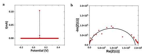
Fig. 7 Electrochemical analyses on an Al(-)/HfO<sub>2</sub>/Cu(+) cell; (a) cyclic voltammetry CV (2 mV s<sup>-1</sup>)  $V_{\rm OC}$  = 0.098 V and (b) electrical impedance spectroscopy EIS performed after the experiment in Fig. 6b with measured  $V_{\rm OC}$  = 0.709 V.
