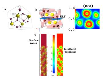
Fig. 2 Structure of hafnium oxide (monoclinic phase  $P2_1/c$ ); (a) crystalline structure; (b) electron localization function (ELF) of a (001) slice; ELF = 1 and ELF =  $\frac{1}{2}$  corresponding to the localized and electron gas; (c) total local potential of a surface (001) of HfO<sub>2</sub>.
