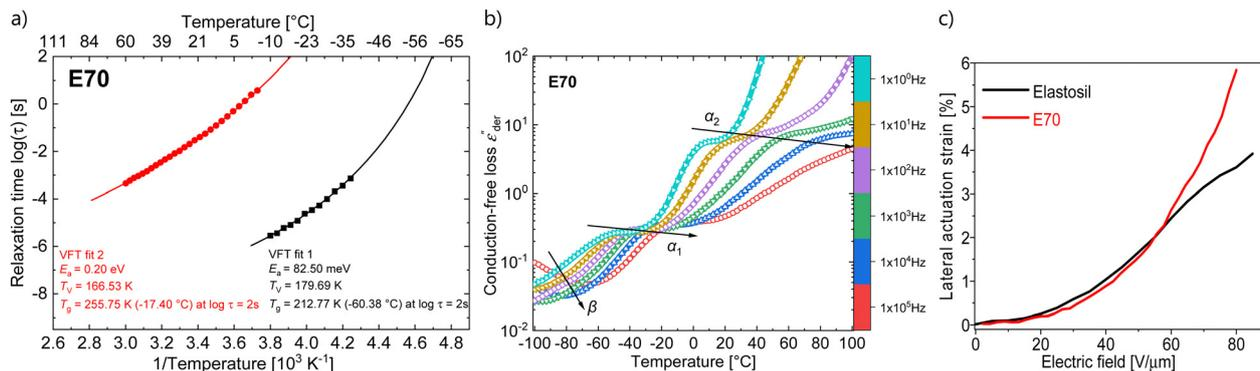
Fig. 5 Arrhenius relaxation plot with VFT fits for samples **E70** (a); isochronal representation of the conduction-free dielectric loss ( $\epsilon''_{\text{der}}$ ) calculated for **E70** sample between  $10^{-1}$  Hz and  $10^6$  Hz (b), and lateral actuation strain of **E70** and Elastosil at different electric fields (c).
