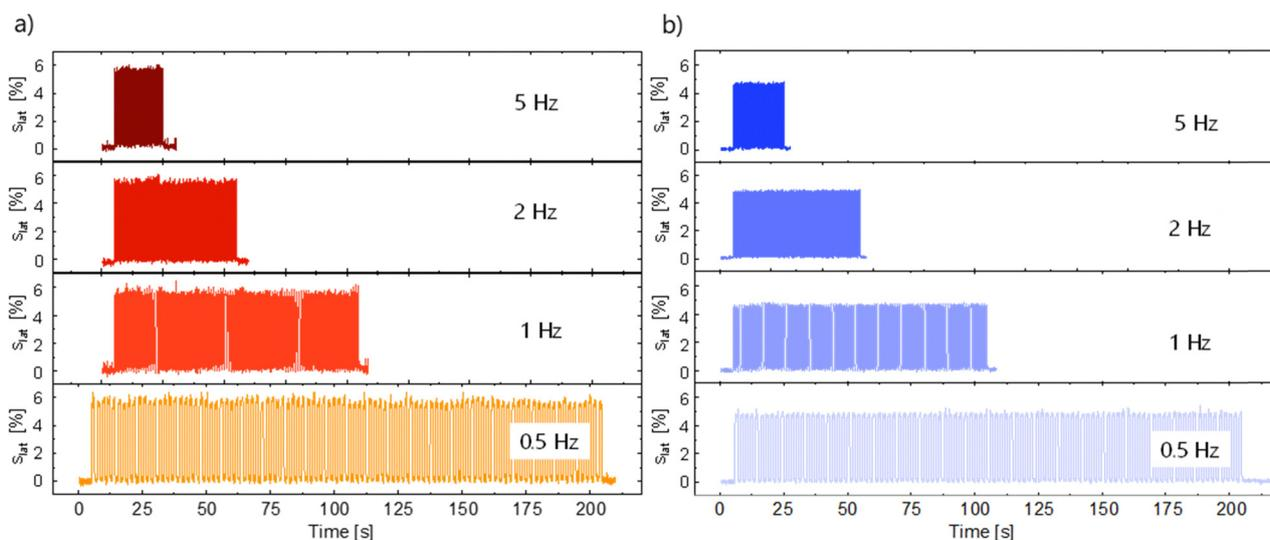
Fig. 6 Lateral actuation strain of **E70** over 100 actuation cycles at 3600 V ( $80 \text{ V } \mu\text{m}^{-1}$ ) (a) and Elastosil at 3640 V ( $85 \text{ V } \mu\text{m}^{-1}$ ) at frequencies from 0.5 Hz to 5 Hz (b).
