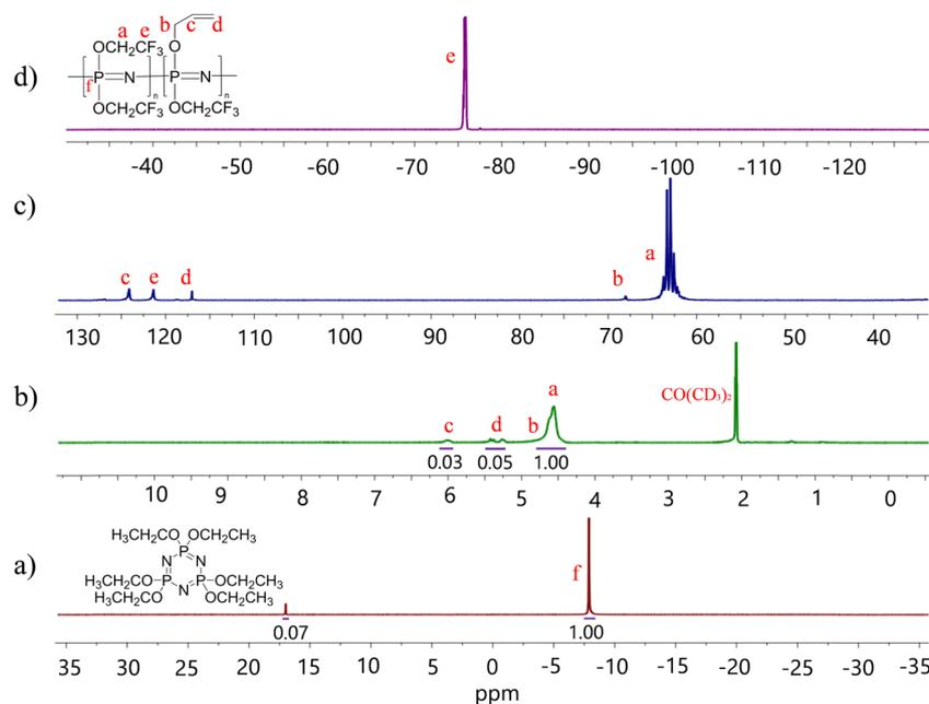
**Fig. 2**  $^{31}\text{P}$  (a);  $^1\text{H}$  (b);  $^{13}\text{C}$  (c);  $^{19}\text{F}$  NMR (d) spectra of the allyl alkoxide substituted poly[bis(2,2,2-trifluoroethoxy)phosphazene] in  $(\text{CD}_3)_2\text{CO}$  at room temperature.
