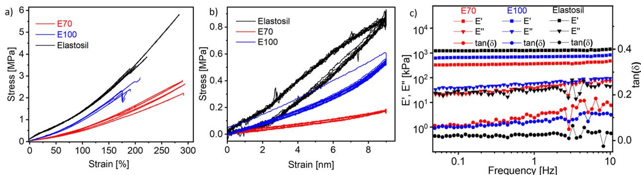
**Fig. 3** Stress-strain curves of **E70**, **E100**, and Elastosil (a). For each material, at least five specimens were tested. Overview of the ten cycles of uniaxial cyclic tensile curves at strains between 0 and 50% **E70**, **E100**, and Elastosil (b). Results for dynamic-mechanical analysis (DMA) of the films **E70** and **E100** (c) at different frequencies, 2% strain, and room temperature.
