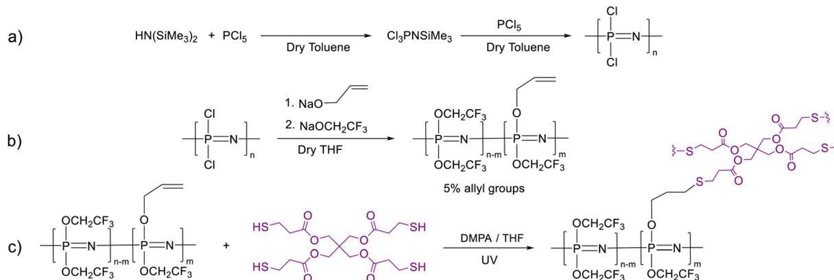
**Scheme 1** Synthesis of the monomer starting from hexamethyldisilazane and  $\text{PCl}_5$  and its polymerization using a  $\text{PCl}_5$  initiator (a); functionalization with trifluoroethoxide and 5 mol% allyl alkoxide groups (b); and cross-linking with pentaerythritol tetrakis(3-mercaptopropionate) via a thiol-ene reaction under UV light using DMPA initiator (c).
