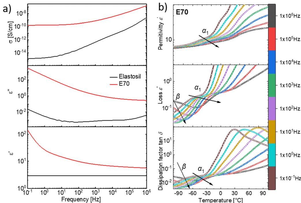
Fig. 4 The conductivity ( $\sigma$ ), loss tangent ( $\tan \delta$ ), dielectric loss ( $\epsilon''$ ), and dielectric permittivity ( $\epsilon'$ ) at room temperature as a function of frequency ranging from 10<sup>-1</sup> and 10<sup>6</sup> Hz of **E70** and Elastosil (a) and dielectric permittivity, permittivity loss, and dissipation factor  $\tan \delta$  of **E70** from -100 to 100 °C at different frequencies (b).
