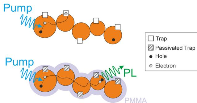
**Scheme 1** Proposed picture for carrier recombination and the role of deep traps. (top) For bare QD films carriers generated in a given QD rapidly recombine non-radiatively at a trap within the same or an adjacent QD. (bottom) Upon passivation of the surface traps, carriers can diffuse across the QD film before recombining.
