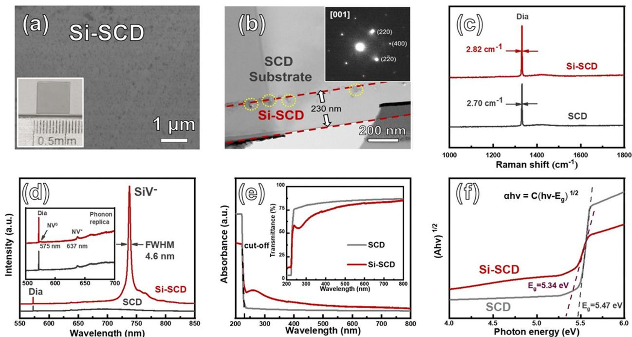
Fig. 2 Plan-view SEM image (a) and TEM cross-section image (b) of the Si-doped SCD sample. Room temperature Raman spectra (c), PL spectra (d), UV-vis absorption/transmittance spectra (e) and the corresponding Tauc plot (f) of the samples.
