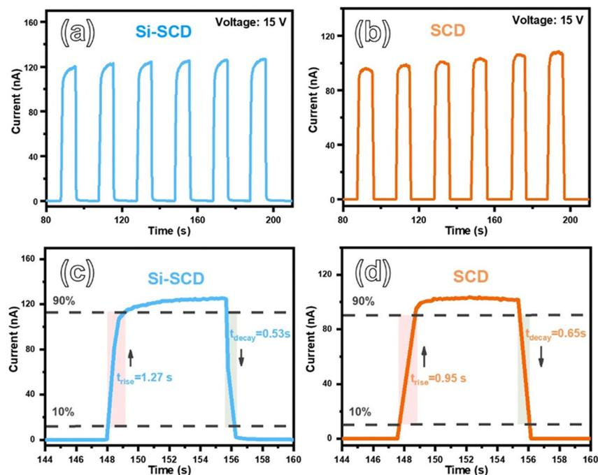
Fig. 5 Time-resolved photocurrent of the Si-doped (a) and (c) and the undoped (b) and (d) SCD detectors.
