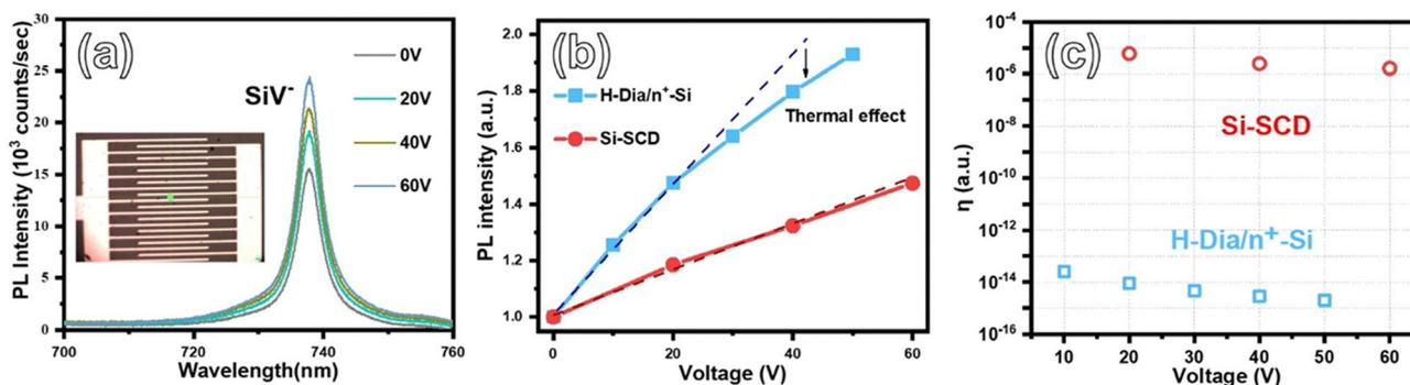
Fig. 6 (a) PL spectra (532 nm laser) of the Si-doped SCD device at different bias voltages. The normalized SiV<sup>-</sup> PL variation (b) and the calculated electrical enhancement efficiency at different bias voltages (c).
