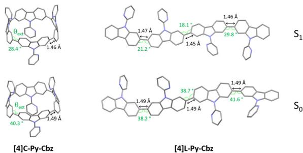
Fig. 5 Optimized geometries (B3LYP/6-31+g(d)):  $S_0$  (ground state, bottom) and  $S_1$  (first singlet excited state, top) of [4]C-Py-Cbz (left) and [4]L-Py-Cbz (right). On each structure, in the  $S_0$  and  $S_1$  states, the modeled mean torsion angle  $\theta_{\text{ext}}$  between the carbazoles and the length of the C-C bond linking two carbazoles are presented.
