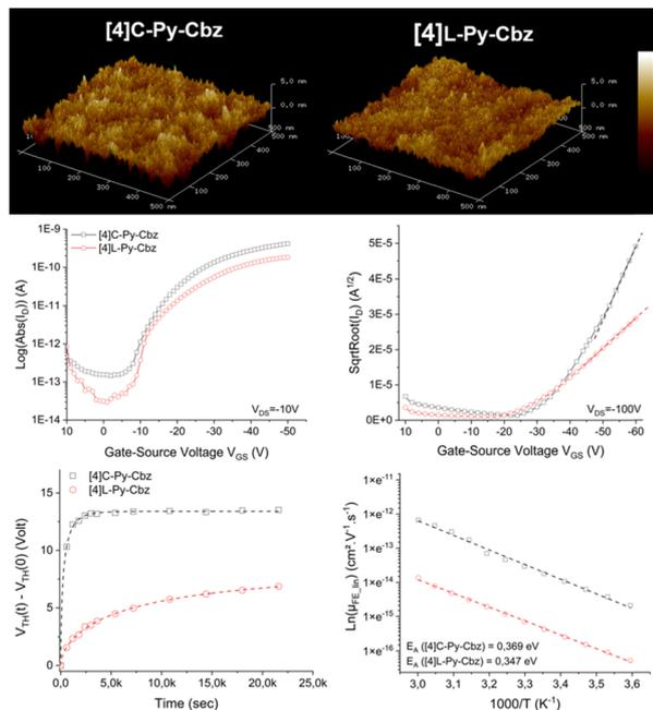
Fig. 6 [4]C-Py-Cbz and [4]L-Py-Cbz top: 2D (500 × 500 nm<sup>2</sup>) AFM images of semiconducting layer deposited under vacuum on SU8 insulating layer, middle: transfer characteristics in linear (left) and saturated (right) regimes. Bottom: Threshold voltage behavior under gate bias stress (V<sub>GS</sub>Stress = -20 V, V<sub>DS</sub>Stress = -10 V) (left) and Arrhenius plots of FE mobility ln(μ<sub>FE</sub>) as a function of 1000/T (right).
