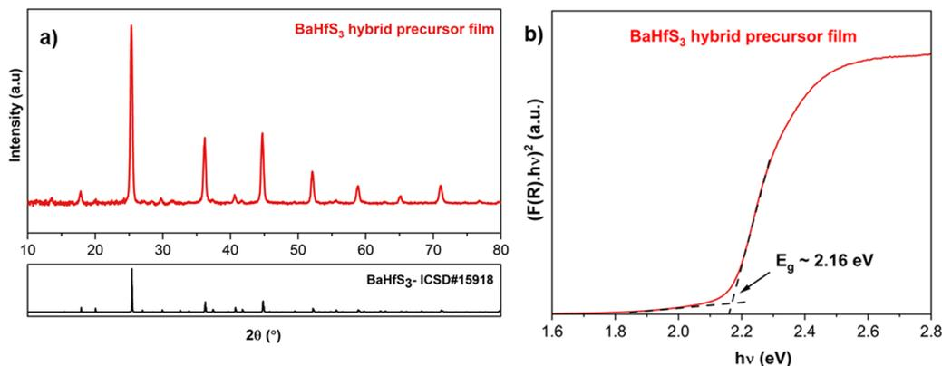
Fig. 7 (a) X-ray diffraction pattern of the BaHfS<sub>3</sub> film obtained after sulfurizing the as-coated BaS–HfS<sub>3</sub> film from the hybrid precursor route. (b) Kubelka–Munk transformation applied to the diffuse reflectance spectra of the BaHfS<sub>3</sub> film derived from hybrid precursor film (considering direct bandgap).<sup>8</sup>
