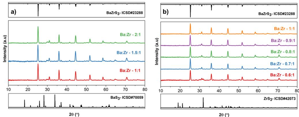
Fig. 1 (a) and (b) X-ray diffraction pattern of the Ba–Zr–S powder synthesized with different Ba:Zr ratios at 575 °C for 12 h with a sulfur pressure of 0.79 atm. BaS and ZrS<sub>2</sub> were used as barium and zirconium precursors. The synthesized powders in (a) were water-washed to remove any water-soluble impurities (BaS<sub>3</sub>). The sample with Ba:Zr 0.6 : 1 in (b) has ZrS<sub>3</sub> impurities.
