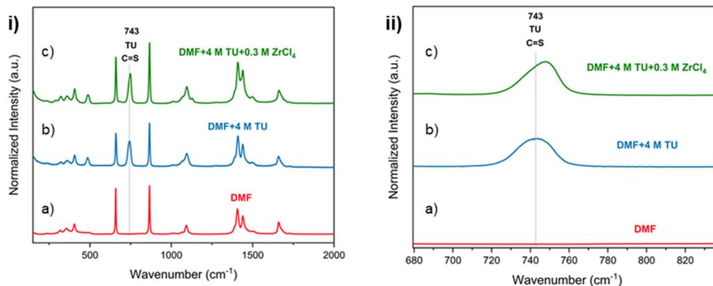
Fig. 3 Liquid Raman on only (a) dimethyl formamide (DMF), (b) thiourea (TU) + DMF, and (c) TU + DMF +  $ZrCl_4$  (0.3 M). The peak shift in the C=S bond stretch of TU suggests a metal–sulfur interaction. (ii) presents the zoomed-in representation of (i).
