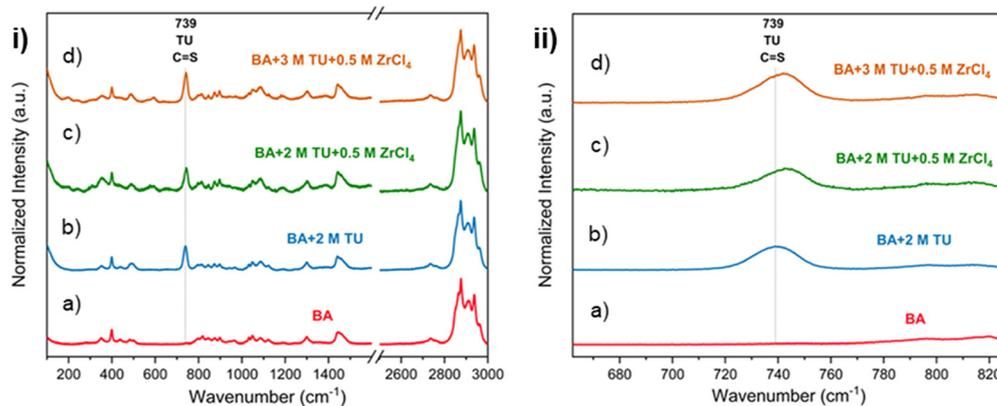
Fig. 4 Liquid Raman on only (a) butylamine (BA), (b) thiourea (TU) + BA, (c) TU (2 M) + BA +  $ZrCl_4$  (0.5 M), and (d) TU (3 M) + BA +  $ZrCl_4$  (0.5 M). The peak shift in the C=S bond stretch of TU suggests a metal–sulfur interaction. (ii) presents the zoomed-in representation of (i).
