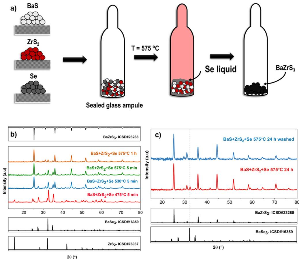
Fig. 8 (a) Reaction schematic depicting the synthesis of BaZrS<sub>3</sub> utilizing a selenium liquid flux. (b) X-ray diffraction patterns illustrating the evolution of intermediate phases with temperature for binary sulfides when subjected to the selenium liquid flux. (c) Comparison plot of the X-ray diffraction pattern for the water-washed and unwashed BaZrS<sub>3</sub> powder.
