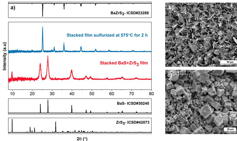
Fig. 5 (a) X-ray diffraction pattern showcasing the as-annealed stacked bilayer film of  $ZrS_3$  and BaS before ampule sulfurization and the  $BaZrS_3$  film after sulfurization. (b) SEM top-view image depicting the  $ZrS_3$  film prepared from the  $ZrCl_4$ –butylamine– $CS_2$ –pyridine solution chemistry. (c) SEM top-view image illustrating the  $BaZrS_3$  film derived from the  $ZrS_3$ –BaS bilayer stack.
