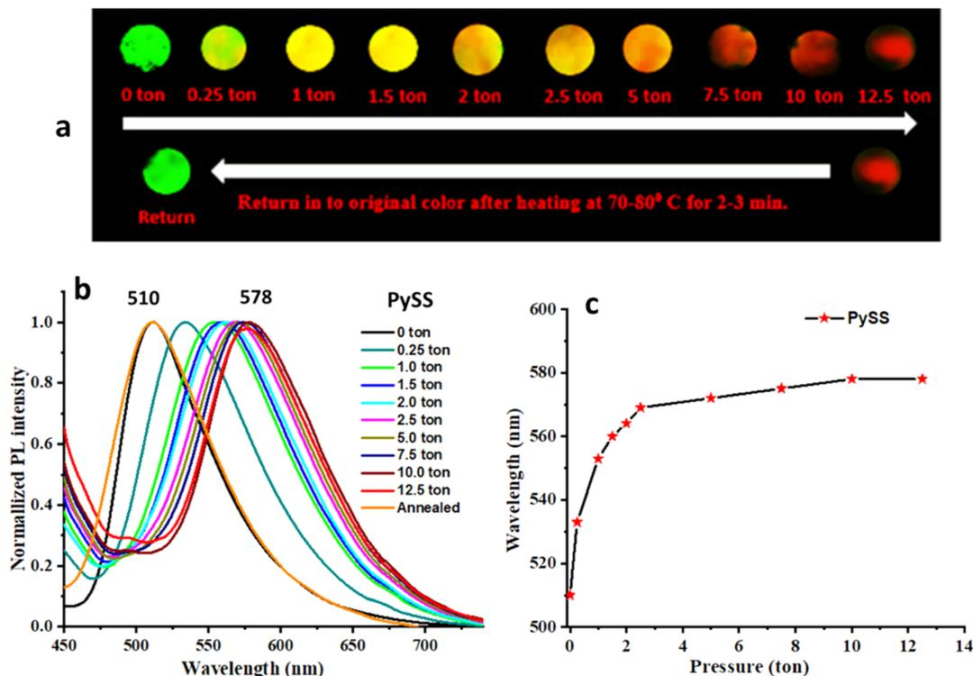
Fig. 6 PL properties of **PySS** under different amounts of hydraulic pressure. (a) Emission images of **PySS** taken under UV excitation (365 nm) with increasing pressure and after releasing pressure; (b) normalized PL spectra of **PySS** at different amounts of pressure; (c) the plot showing the change in wavelength at different amounts of pressure.
