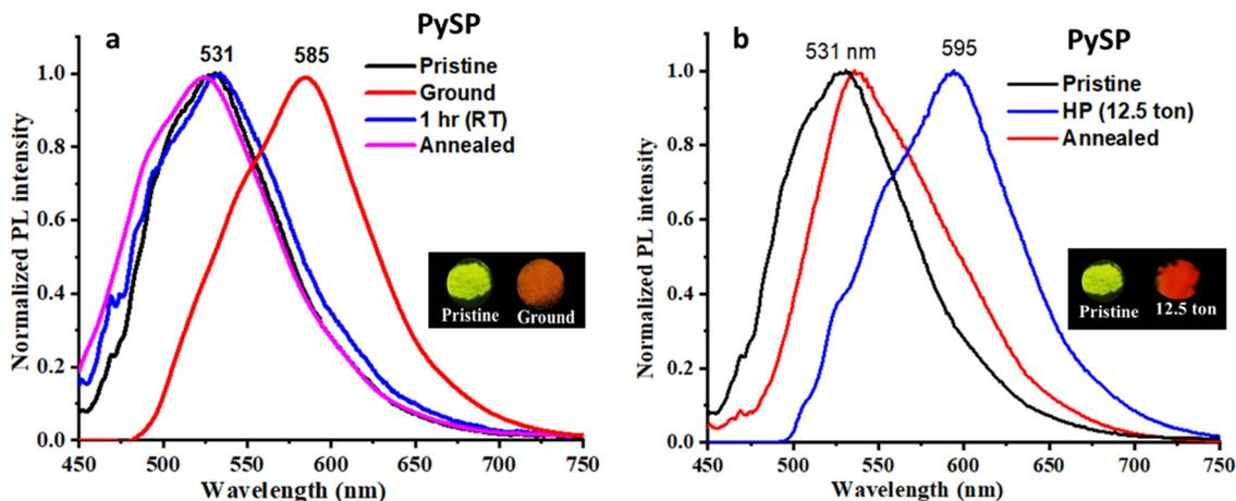
Fig. 5 (a) PL spectra of **PySP** in the pristine form and after grinding with the help of a mortar and pestle. 1 h (RT) indicates that the ground sample was kept for 1 h at RT and the emission was recorded. (b) PL spectra of **PySP** after applying hydraulic press (HP) of 12.5 ton and heating at 70–80 °C for 1–2 min (annealed sample).
