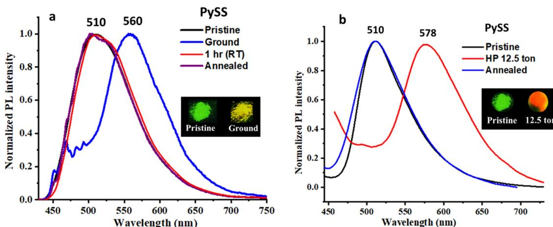
Fig. 4 (a) PL spectra of **PySS** in the pristine form and after grinding with the help of a mortar and pestle; 1 h (RT) indicates that the ground sample was kept for 1 h at rt and then the emission was recorded. (b) PL spectra of **PySS** after applying hydraulic press (HP) of 12.5 ton and heating at  $70\text{--}80^\circ\text{C}$  for 1–2 minutes (annealed sample).
