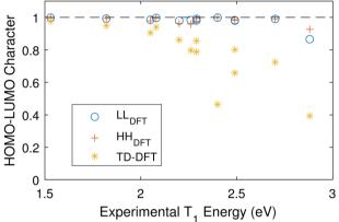
Fig. 5 (a) Calculated vertical triplet energies as a function experimental values. Both DFT and TD-DFT were carried out at the optimized S<sub>0</sub> geometry using B3LYP/cc-pVTZ. The DFT systematically overestimates the value of the triplet. (b) The HOMO-LUMO character of the  $S_0$  to  $T_0$ transition as output by TD-DFT and estimated using eqn (5) for DFT.
