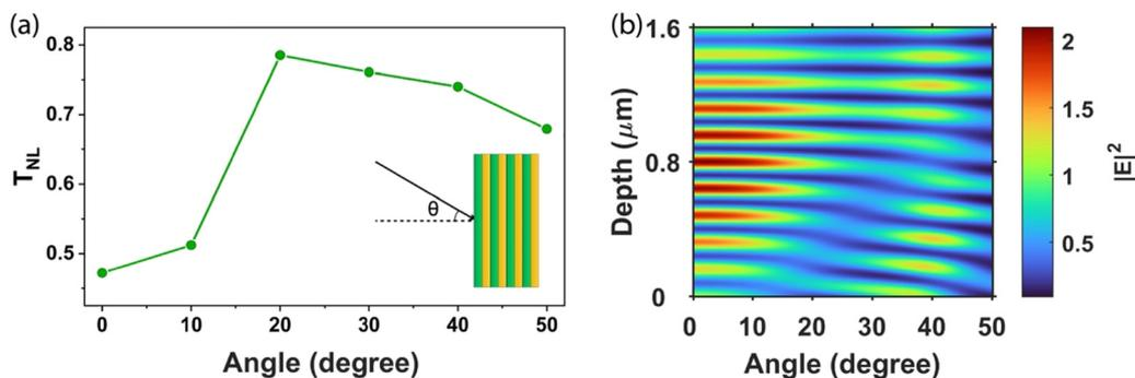
Fig. 5 (a)  $T_{\text{NL}}$  (nonlinear transmittance at the focus for the on-axis peak intensity of  $1.4 \times 10^{12} \text{ W m}^{-2}$ ) of PhC at different angles of incidence. (b) Simulated electric field profile in the DBR as a function of external angle of incidences.
