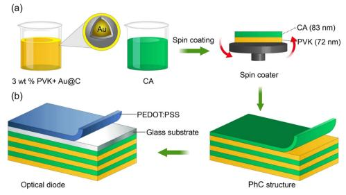
Fig. 2 (a) Fabrication of PhC using the spin coating technique. (b) Schematic of the PEDOT:PSS/PhC optical diode fabricated in this study.
