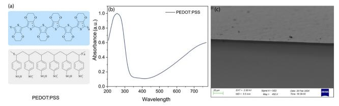
(a) Primary structure of PEDOT:PSS, (b) UV-visible absorption spectrum, (c) cross-sectional SEM.
