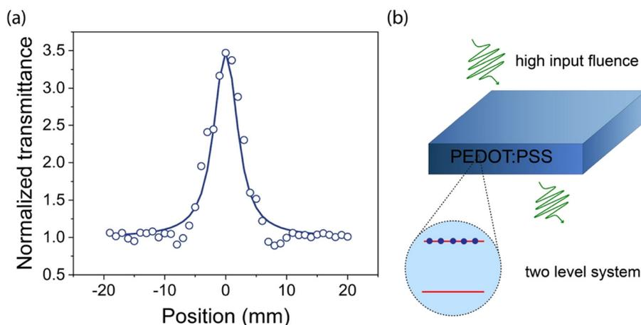
Fig. 7 (a) Normalized transmittance of a pure PEDOT:PSS film as a function of sample position. Experimental data are depicted as circles, while theoretical fits based on eqn (2) are shown as solid lines. (b) Mechanism of saturable absorption.
