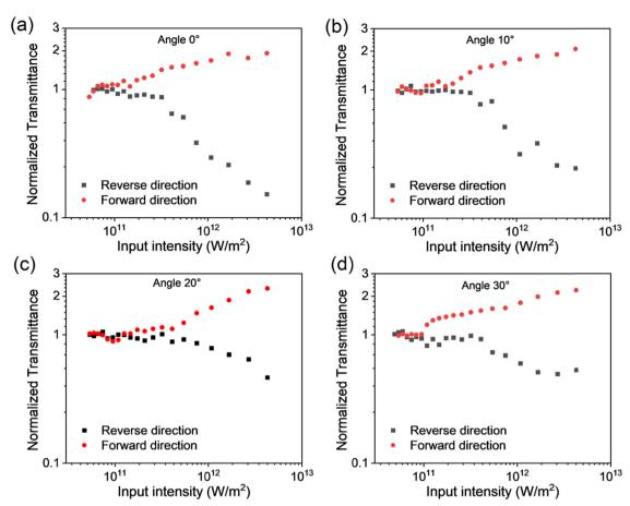
Fig. 9 Transmission characteristics of the PEDOT:PSS/PhC optical diode. Light transmission in forward bias (red circle) and reverse bias (black square). Diode transmission plot for (a) 0°, (b) 10°, (c) 20°, and (d) 30°
