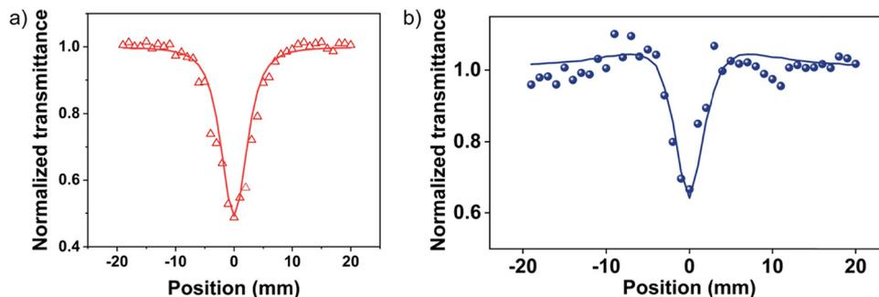
Fig. 4 (a) The open aperture Z-scan data of PhC at the on-axis peak intensity of  $1.4 \times 10^{12} \text{ W m}^{-2}$  and (b) Z-scan data at an on-axis peak intensity of  $7 \times 10^{11} \text{ W m}^{-2}$ .
