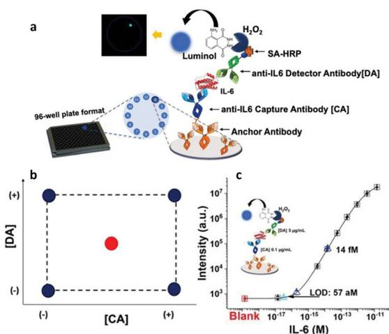
Fig. 5 (a) Workflow of the biosensor development; (b) experimental domain; (c) calibration curve with optimal CA and DA concentrations, such as  $0.1 \mu\text{g mL}^{-1}$  and  $5 \mu\text{g mL}^{-1}$ , respectively. Adapted and reproduced with permission from ref. 34. Copyright 2023, Wiley-VCH under Creative Commons Attribution 4.0 License (CC BY 4.0).
