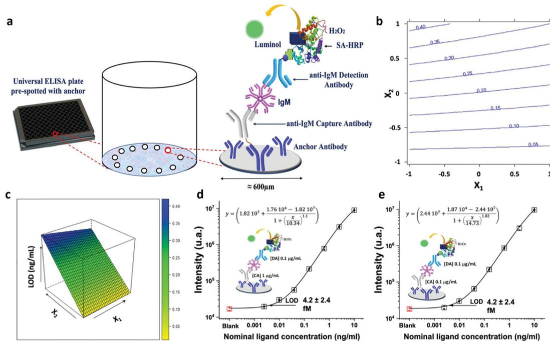
Fig. 4 (a) Scheme of the biosensor development; (b) isoresponse contour plot and (c) the response surface for LOD response. IgM calibration curve recorded using (d)  $1\ \mu\text{g mL}^{-1}$  and  $0.1\ \mu\text{g mL}^{-1}$  and (e)  $0.1\ \mu\text{g mL}^{-1}$  and  $0.1\ \mu\text{g mL}^{-1}$  of CA and DA anti-IgM antibodies respectively. Adapted and reproduced with permission from ref. 35. Copyright 2022, Wiley-VCH under Creative Commons Attribution 4.0 License (CC BY 4.0).
