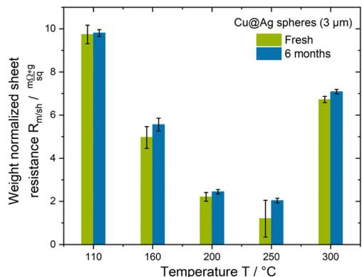
Fig. 6 Stability of weakly sintered prints under ambient conditions.  $R_{m/sh}$  of prints containing 3  $\mu\text{m}$ -sized Cu@Ag-S after sintering ('fresh') and after 6 months storage in laboratory air at standard conditions (cf. Preparation and printing of pastes.).
