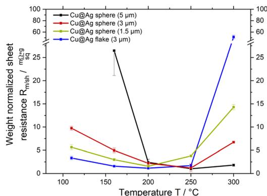
Fig. 1 Weight-normalized sheet resistances  $R_{m/sh}$  of printed films of silver-copper core-shell particles after 30 min in air at temperature  $T$ . All particles contained 10 wt% of silver as shells. Spherical particles had average diameters of 1.5, 2.5, 5  $\mu\text{m}$ . Flakes had an equivalent average diameter of 3  $\mu\text{m}$ .
