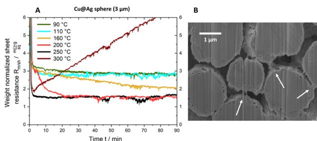
Fig. 4 (A) Resistance evolution of prints and (B) micro-structural changes at 200 °C. (A)  $R_{m/sh}$  as measured *in situ* while treating different prints of 3  $\mu$ m sized Cu@Ag-S treated at 90 °C to 300 °C for 90 min. The measurement started at 0 min when placing the sample on a preheated hot plate. (B) Electron microscopy of a cross-section prepared from a sample treated at 200 °C indicated silver necks (white arrows).
