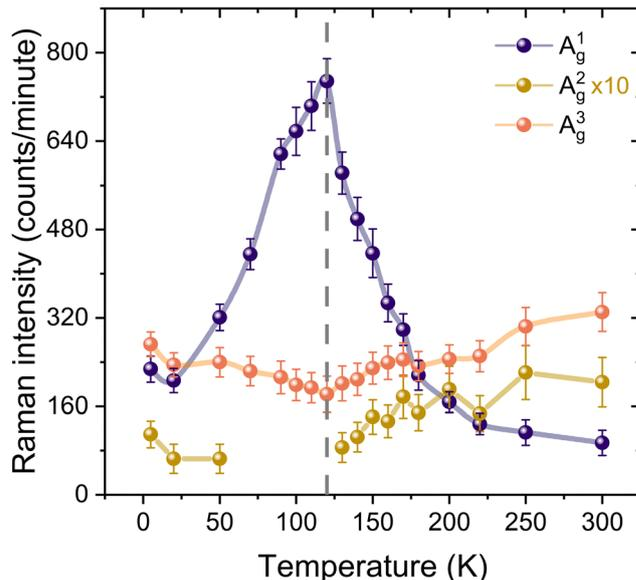
**Fig. 3** The Stokes Raman spectral intensities, as a function of temperature, of the  $A_g^1$ ,  $A_g^2$ , and  $A_g^3$  modes. From 125 K down to 70 K, the  $A_g^2$  mode exhibits zero intensity due to complete suppression. The vertical dashed line indicates 120 K.
