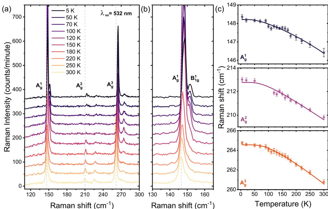
Fig. 2 (a) and (b) Temperature-dependent Raman spectra of bulk PdSe<sub>2</sub> under parallel configuration (xx), with an excitation energy of 2.33 eV (532 nm). (c) Raman frequencies as a function of temperature for the  $A_g^1$ ,  $A_g^2$ , and  $A_g^3$  phonon modes. In each panel, we fit the data to the anharmonic model characterized by the processes of optical phonon decay (solid lines) using eqn (1) over the entire temperature range 5 to 300 K.
