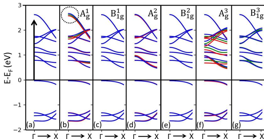
Fig. 7 Estimating the electron–phonon coupling using DFT calculations for the electronic dispersion of bulk PdSe<sub>2</sub> considering (a) unperturbed (green lines) and (b–g) different frozen phonons (blue and red for opposite displacements) (b) A<sub>g</sub><sup>1</sup>, (c) B<sub>1g</sub><sup>1</sup>, (d) A<sub>g</sub><sup>2</sup>, (e) B<sub>1g</sub><sup>2</sup>, (f) A<sub>g</sub><sup>3</sup>, and (g) B<sub>1g</sub><sup>3</sup>.
