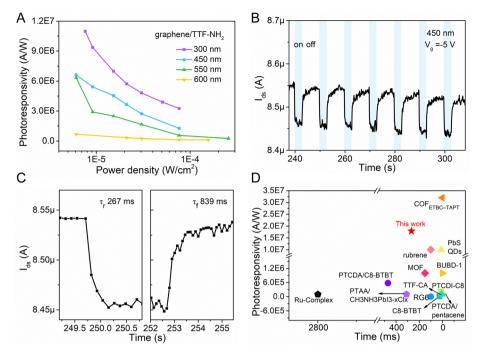
Fig. 4 (A) Photoresponsivity of the graphene/TTF-NH2 transistor at different wavelengths. (B) and (C) Temporal photocurrent of the graphene/TTF-NH<sub>2</sub> transistor under dark and 450 nm irradiation conditions, and the corresponding transfer curves are shown in Fig. S10B (ESI†). (D) Comparison of the photoresponsivity and response time performance of this work (graphene/TTF-NH<sub>2</sub>) with reported graphene-based photodetectors.
