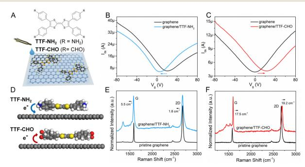
Fig. 1 (A) Schematic diagram of physisorption of TTF molecules onto exfoliated graphene. Transfer characteristics of pristine graphene and graphene assembled with (B) TTF-NH2 and (C) TTF-CHO in the dark. (D) Schematics of charge transfer between TTF derivatives and the graphene system based on theoretical calculations. Raman spectra of pristine graphene, (E) graphene/TTF-NH2 and (F) graphene/TTF-CHO hybrids.
