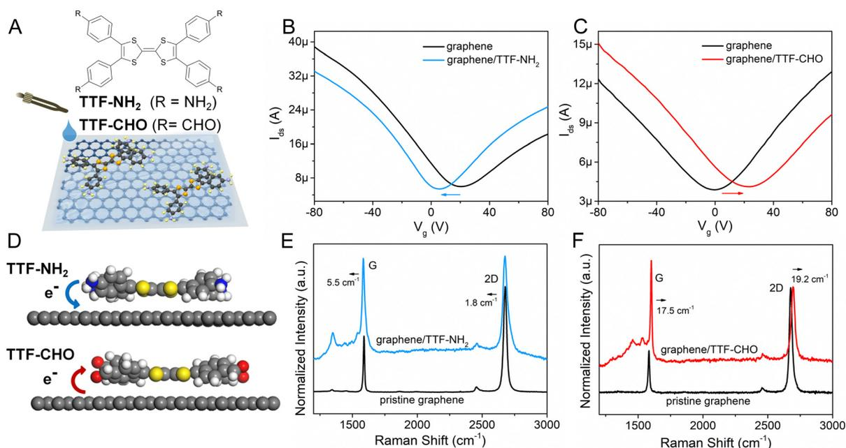
Fig. 1 (A) Schematic diagram of physisorption of TTF molecules onto exfoliated graphene. Transfer characteristics of pristine graphene and graphene assembled with (B) TTF-NH<sub>2</sub> and (C) TTF-CHO in the dark. (D) Schematics of charge transfer between TTF derivatives and the graphene system based on theoretical calculations. Raman spectra of pristine graphene, (E) graphene/TTF-NH<sub>2</sub> and (F) graphene/TTF-CHO hybrids.
