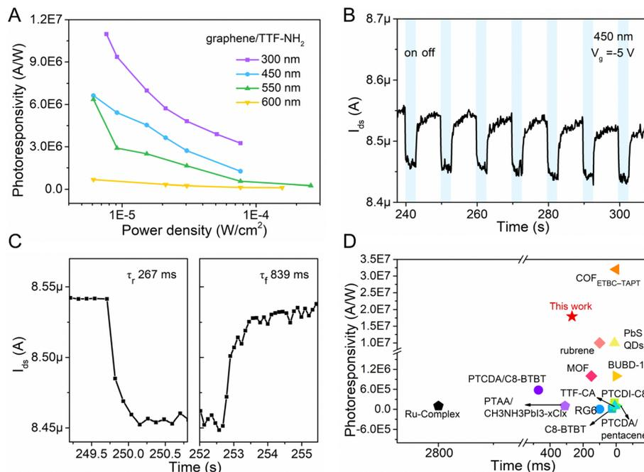
Fig. 4 (A) Photoresponsivity of the graphene/TTF-NH<sub>2</sub> transistor at different wavelengths. (B) and (C) Temporal photocurrent of the graphene/TTF-NH<sub>2</sub> transistor under dark and 450 nm irradiation conditions, and the corresponding transfer curves are shown in Fig. S10B (ESI<sup>†</sup>). (D) Comparison of the photoresponsivity and response time performance of this work (graphene/TTF-NH<sub>2</sub>) with reported graphene-based photodetectors.
