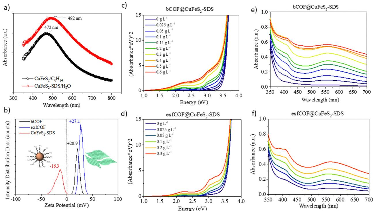
**Fig. 2** (a) UV-vis absorption of  $\text{CuFeS}_2\text{-OP}$  and  $\text{CuFeS}_2\text{-SDS}$ . (b) Zeta potential of the bCOF, exfCOF and the  $\text{CuFeS}_2\text{-SDS}$  in water. (c) and (d) The Tauc plots of hybrid materials, depicting the increased absorption in the visible light range after the incorporation by increasing weight of the plasmonic nanoparticles in  $0.2 \text{ g L}^{-1}$  bCOF and  $0.2 \text{ g L}^{-1}$  exfCOF and (e) and (f) their corresponding UV-visible spectra.
