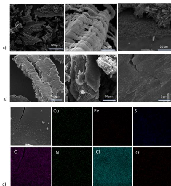
Fig. 3 SEM images of the (1–1) (a) bCOF@CuFeS<sub>2</sub>-SDS and (b) exfCOF@CuFeS<sub>2</sub>-SDS hybrid materials. (c) EDX mapping of the Cu, Fe, and S elements of the nanoparticles on bCOF@CuFeS<sub>2</sub>-SDS.
