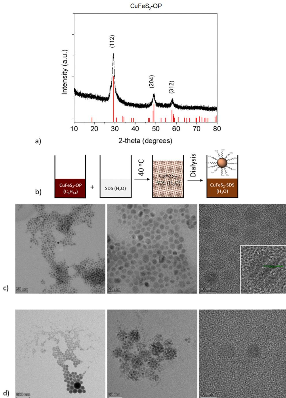
**Fig. 1** (a) XRD pattern of the as made  $\text{CuFeS}_2\text{-OP}$  nanoparticles. (b) Schematic representation of the solubilization process of  $\text{CuFeS}_2\text{-OP}$  to  $\text{CuFeS}_2\text{-SDS}$  (c) TEM images of the organophilic nanoparticles dispersed in hexane ( $\text{CuFeS}_2\text{-OP}$ ), along with the HRTEM of the nanoparticles' planes and (d) the hydrophilic functionalized nanoparticles dispersed in water ( $\text{CuFeS}_2\text{-SDS}$ ).
