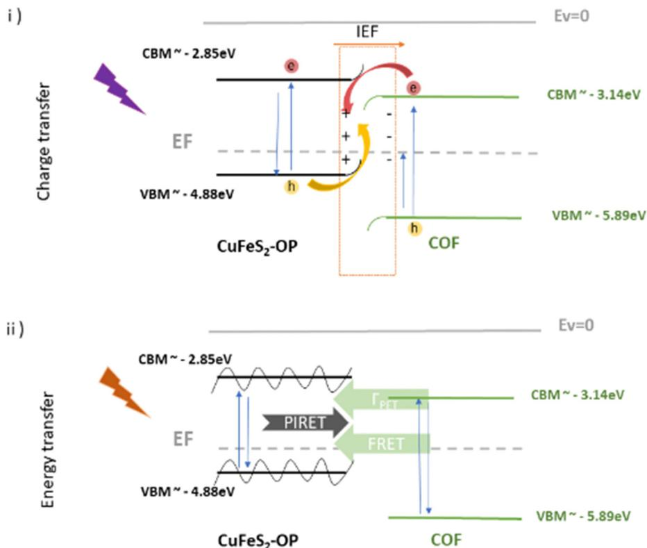
**Scheme 1** Schematic representation of the band energy positions of CuFeS<sub>2</sub>-OP nanoparticles and the COF, along with the proposed transfer mechanisms after contact and under (i) UV and (ii) visible illumination at the S-scheme.
