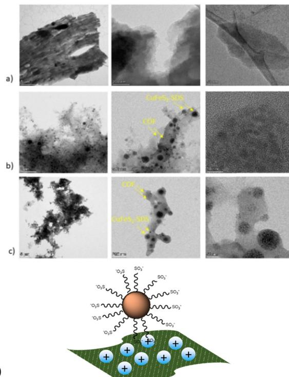
Fig. 4 TEM images of (a) bCOF, (b) (1–1) bCOF@CuFeS<sub>2</sub>-SDS and (c) (1–1) exfCOF@CuFeS<sub>2</sub>-SDS (d) and a schematic representation of the as-formed hybrids.
