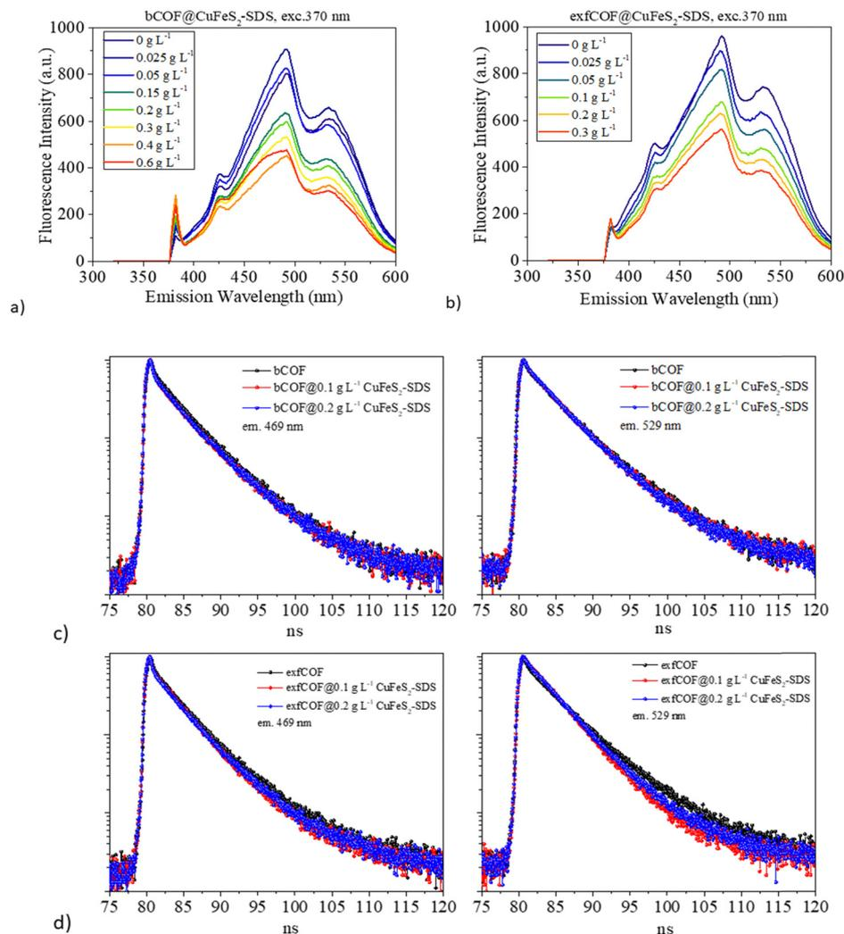
Fig. 5 (a) and (b) Steady-state photoluminescence of the 0.2 g L<sup>-1</sup> bCOF and 0.2 g L<sup>-1</sup> exfCOF and their hybrid materials. (c) Time-resolved fluorescence for 0.2 g L<sup>-1</sup> bCOF, bCOF@CuFeS<sub>2</sub>-SDS and (d) 0.2 g L<sup>-1</sup> exfCOF, exfCOF@CuFeS<sub>2</sub>-SDS after the addition of 0.1 and 0.2 g L<sup>-1</sup> CuFeS<sub>2</sub>-SDS at  $\lambda_{\text{em}} = 469$  & 529 nm.
