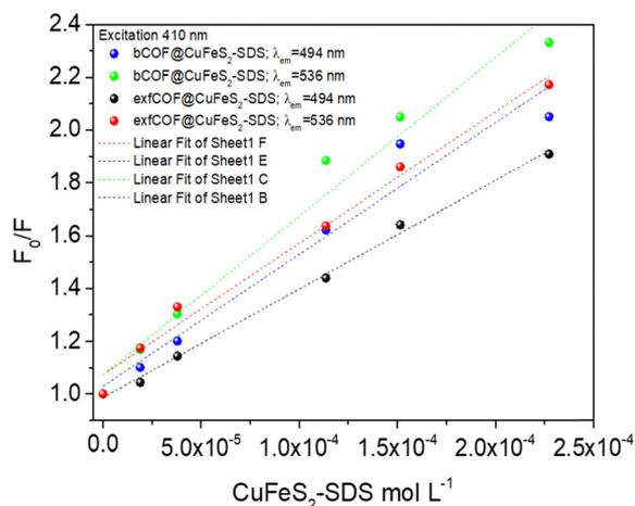
**Fig. 6** The Stern–Volmer ( $F_0/F$ ) plots at 494 nm and 536 nm emissions of bCOF@CuFeS<sub>2</sub>-SDS and exfCOF@CuFeS<sub>2</sub>-SDS under steady-state excitation of  $\lambda_{\text{exc}} = 410$  nm.
