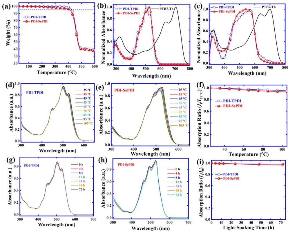
Fig. 1 TG curve for asymmetric acceptors **PDI-TPDI** and **PDI-SePDI** (a), absorption in dilute  $\text{CH}_2\text{Cl}_2$  (b) and as neat films (c), temperature-dependent absorption for **PDI-TPDI** (d) and **PDI-SePDI** (e) as well as the curve of maximum absorption intensity relative to temperature (f), changes for UV-vis absorption for **PDI-TPDI** (g) and **PDI-SePDI** (h) in chlorobenzene after illumination, and absorption intensity variation trend relative to light-soaking time (i).
