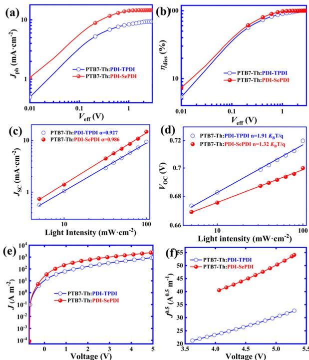
Fig. 5 Plots of  $J_{ph}$  vs. effective voltage ( $V_{eff}$ ) (a),  $\eta_{diss}$  vs.  $V_{eff}$  (b),  $J_{sc}$  vs. light intensity (c),  $V_{oc}$  vs. light intensity (d),  $J$ - $V$  curve (e) and fitting  $J^{0.5}$ - $V$  curve (f) for **PDI-TPDI** and **PDI-SePDI**-based devices.
