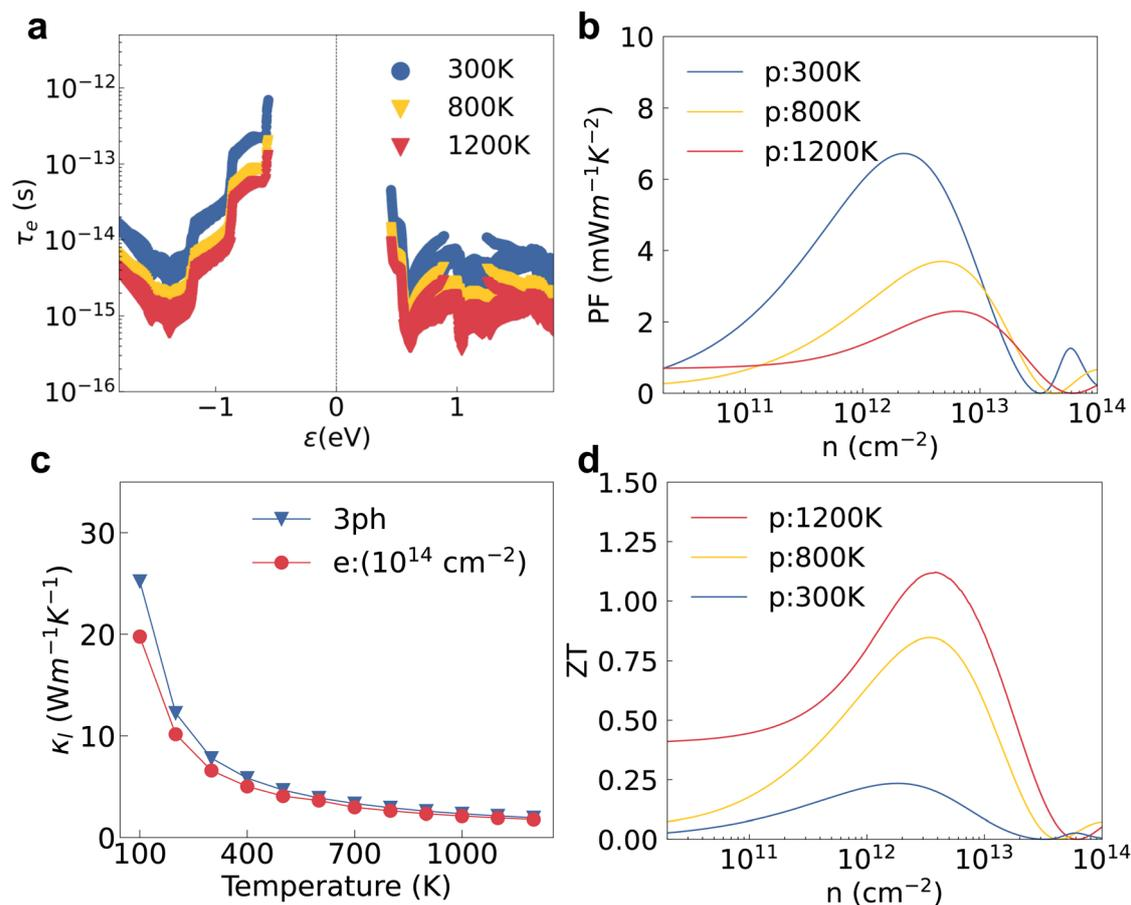
Fig. 5 (a) The electron relaxation time, (b) the power factor under p-type doping, (c)  $\kappa_l$  of the undoped structure and the  $\kappa_l$  values at an electron concentration of  $10^{14} \text{ cm}^{-2}$ , and (d) the final p-type ZT results at different temperatures.
