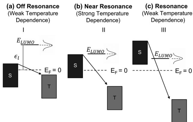
Fig. 3 Energetic landscape of charge transport in a molecular junction governed by eqn (3) when LUMO is the orbital responsible for facilitating transport.  $\epsilon_L$  represents the energetic position of LUMO, which is placed off resonance in panel (a), near resonance in (b), and in resonance (c).
