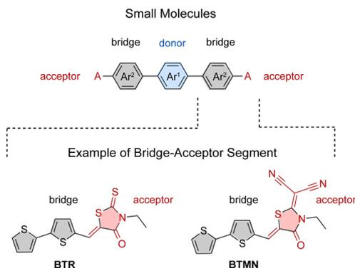
Fig. 1 Schematic representation of the molecular structure of small molecule semiconductors (top). Selected representative examples of the bridge–acceptor molecular structure segment (bottom). **BTR** = bithiophene vinyl rhodanine; **BTMN** = bithiophene vinyl rhodanine malonitrile.
