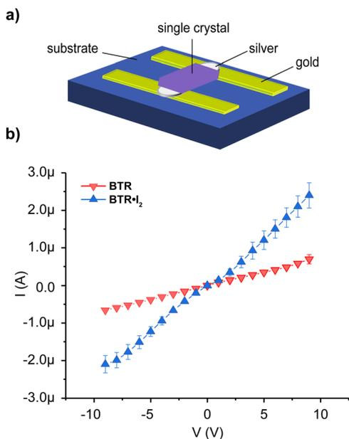
Fig. 5 (a) Device architecture for single-crystal electrical characterization. (b) Average current–voltage plots of **BTR** (red) and **BTR·I<sub>2</sub>** (blue).
