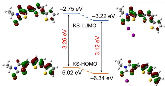
Fig. 4 Kohn–Sham frontier orbital energy levels for **BTR** (left) and **BTR·I<sub>2</sub>** (right). Color: carbon, gray; nitrogen, blue; oxygen, red; sulfur, yellow; hydrogen, white. Cutoff value = 0.05 |e|.
