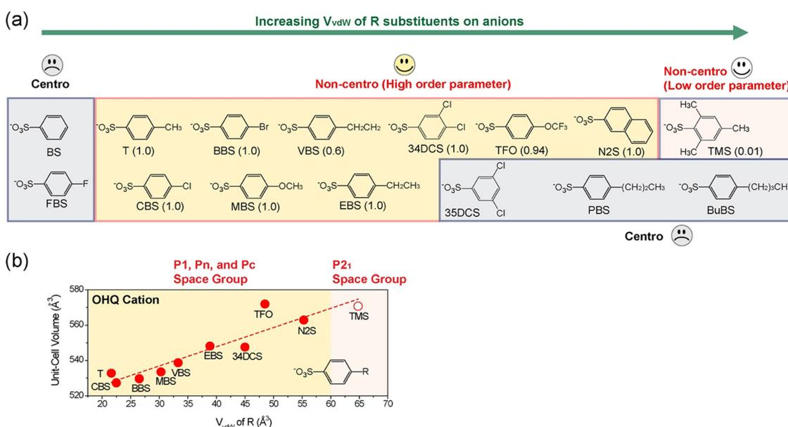
Fig. 5 (a) Schematic trend of the crystal structure characteristics of OHQ-based crystals with various counter anions with different van der Waals volume,  $V_{\text{vdw}}$  of R substituents. (b) The corresponding volume of a cation–anion pair (unit-cell volume divided by the crystallographic Z number) as a function of van der Waals volume,  $V_{\text{vdw}}$  of R substituents. Reproduced and adapted with permission.<sup>74</sup> Copyright 2023, Wiley-VCH.
