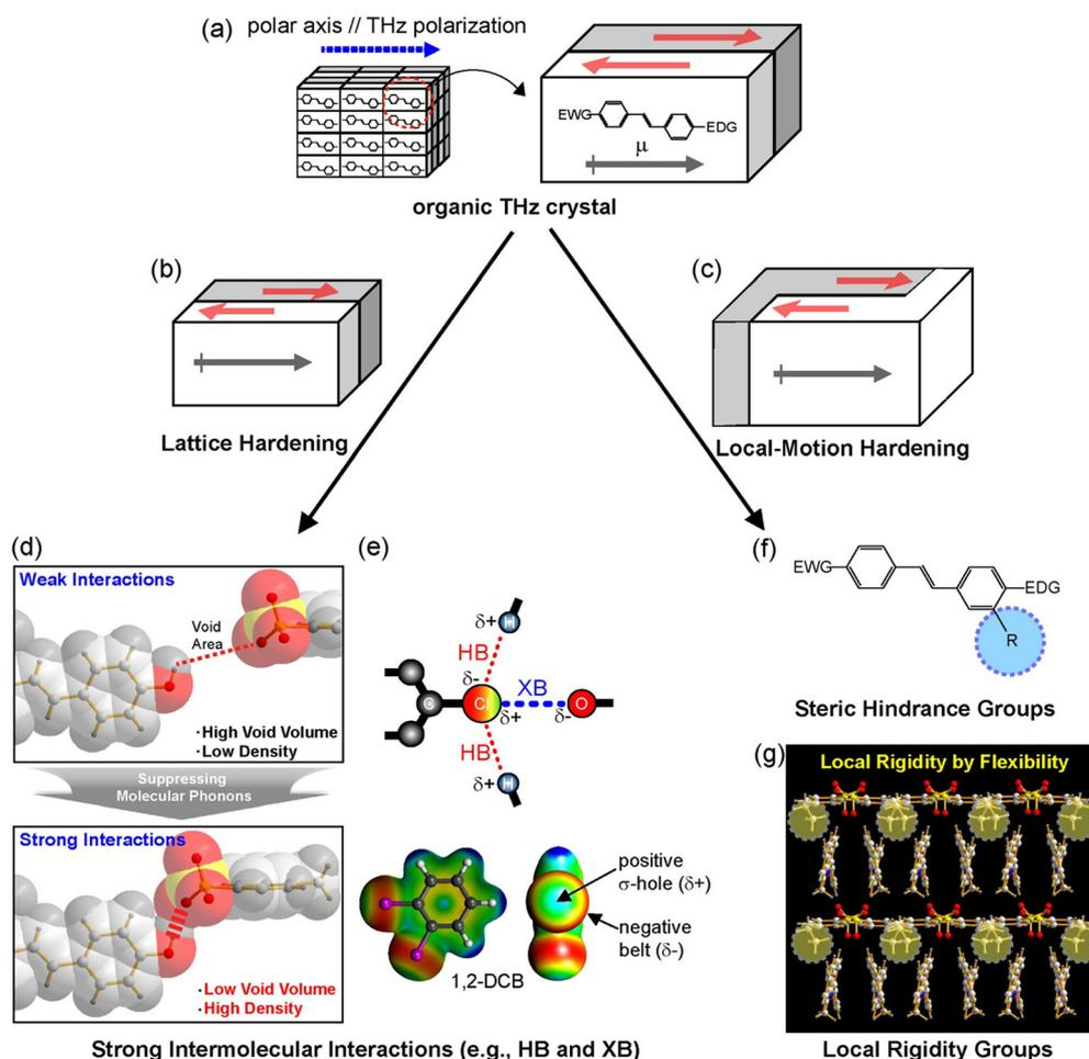
Fig. 6 Schematics of strategies for suppressing phonon vibrations of (a) benchmark organic THz crystals: (b) lattice hardening by (d) and (e) introducing strong intermolecular interaction groups and (c) local-motion hardening by (f) introducing steric hindrance group and (g) local rigidity group with a high conformational freedom. Reproduced and adapted with permission.<sup>55,73,76,77</sup> Copyright 2022 and 2023, Wiley-VCH.
