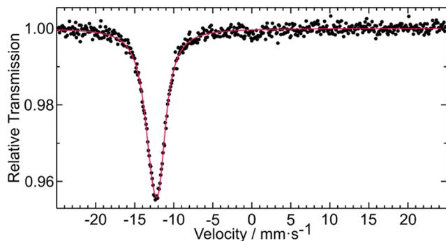
**Fig. 2** Experimental (data points) and simulated (red line) <sup>151</sup>Eu Mössbauer spectrum of EuHfSe<sub>3</sub> measured at 78 K.
