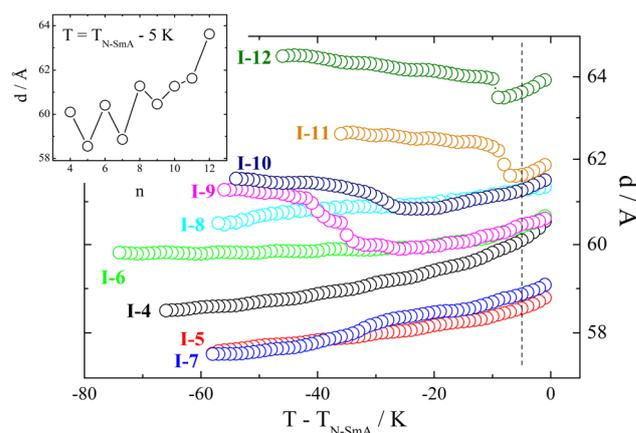
**Fig. 3** Smectic layer thickness,  $d$ , measured as a function of temperature for the studied homologues I- $n$ . In the inset, the layer spacing in the SmA phase, determined 5 K below the Iso-SmA or N-SmA phase transition (dashed line on the main panel), is presented.
