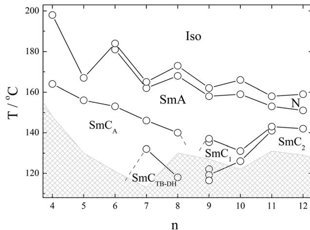
**Fig. 2** Phase diagram of the studied homologues upon elongation of the spacer between the rigid core and the terminal nitrophenyl group. Gray tiled area shows the stability range of the crystal phase marked by melting points.
