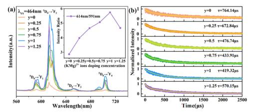
Fig. 4 (a) Photoluminescence emission spectra of  $(KMg)_ySc_{2-y}W_3O_{12}$ :1 mol%  $Eu^{3+}$  (y=0, 0.25, 0.5, 0.75, 1, and 1.25) phosphors, inset: the intensity ratio  $\beta$  with different (KMg)<sup>3+</sup> concentrations. (b) Photoluminescence decay curves of Eu<sup>3+,5</sup>D<sub>0</sub>.
