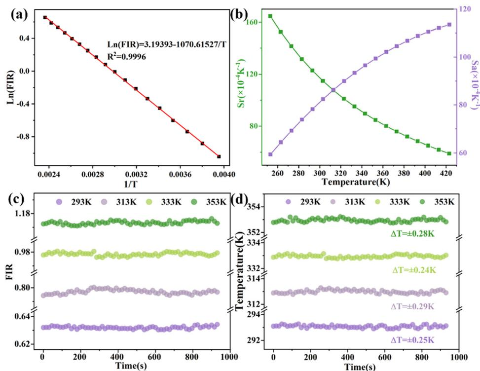
Fig. 9 (a) The relationship between  $\text{Ln}(\text{FIR})$  and  $1/T$ . (b) Absolute sensitivity and relative sensitivity of  $(\text{KMg})\text{ScW}_3\text{O}_{12}$  phosphor dependence on temperature. (c) Calculated FIR values at 293 K, 313 K, 333 K and 353 K. (d) Corresponding temperature and  $\Delta T$  recorded at 293 K, 313 K, 333 K and 353 K.
