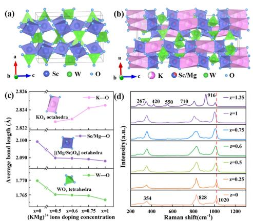
Fig. 2 Crystallographic structure of (a) orthorhombic  $Sc_2W_3O_{12}$  and (b) hexagonal  $(KMg)_xSc_{2-x}W_3O_{12}$ . (c) The influence of  $(KMg)^{3+}$  ion doping on the average bond length of K–O, Mg/Sc–O and W–O bonds. (d) Raman spectra of  $(KMg)_zSc_{2-z}W_3O_{12}$  phosphors
