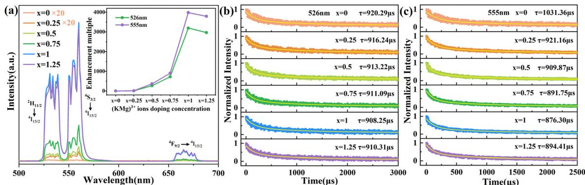
Fig. 5 (a) Upconversion emission spectra of  $(\text{KMg})_x\text{Sc}_{2-x}\text{W}_3\text{O}_{12}:1 \text{ mol}\% \text{Er}^{3+}/20 \text{ mol}\% \text{Yb}^{3+}$  ( $x = 0, 0.25, 0.5, 0.75, 1$ , and  $1.25$ ) phosphors, inset: multiple luminescence enhancement of the phosphor with different  $(\text{KMg})^{3+}$  concentrations. Photoluminescence decay curves of  $\text{Er}^{3+}$ : (b)  ${}^2\text{H}_{11/2}$  and (c)  ${}^4\text{S}_{3/2}$  in phosphors monitored at 370 nm.
