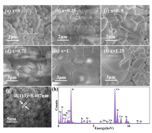
Fig. 3 (a)–(f) SEM images of  $(KMg)_xSc_{2-x}W_3O_{12}:1 \text{ mol}\% \text{ Er}^{3+}/20 \text{ mol}\% \text{ Yb}^{3+}$  (x = 0, 0.25, 0.5, 1, 0.75, and 1.25) phosphors. (g) HRTEM image and (h) EDX results of the (KMg)ScW<sub>3</sub>O<sub>12</sub>:1 mol% Er<sup>3+</sup>/20 mol% Yb<sup>3+</sup> phosphor.
