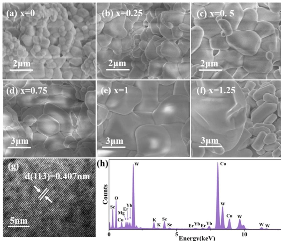
Fig. 3 (a)–(f) SEM images of  $(\text{KMg})_y\text{Sc}_{2-y}\text{W}_3\text{O}_{12}:1 \text{ mol}\% \text{Er}^{3+}/20 \text{ mol}\% \text{Yb}^{3+}$  ( $x = 0, 0.25, 0.5, 1, 0.75,$  and  $1.25$ ) phosphors. (g) HRTEM image and (h) EDX results of the  $(\text{KMg})\text{ScW}_3\text{O}_{12}:1 \text{ mol}\% \text{Er}^{3+}/20 \text{ mol}\% \text{Yb}^{3+}$  phosphor.
