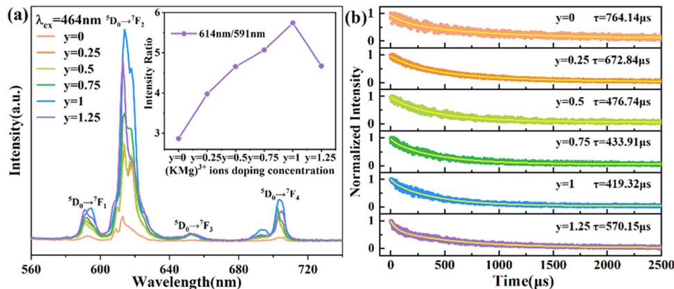
Fig. 4 (a) Photoluminescence emission spectra of  $(\text{KMg})_y\text{Sc}_{2-y}\text{W}_3\text{O}_{12}:1 \text{ mol}\% \text{Eu}^{3+}$  ( $y = 0, 0.25, 0.5, 0.75, 1,$  and  $1.25$ ) phosphors, inset: the intensity ratio  $\beta$  with different  $(\text{KMg})^{3+}$  concentrations. (b) Photoluminescence decay curves of  $\text{Eu}^{3+}:^5\text{D}_0$ .
