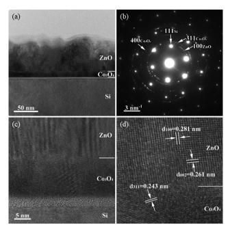
Fig. 2 (a) TEM image at low magnification of the Si/Co<sub>3</sub>O<sub>4</sub>/ZnO structure, (b) corresponding SAED pattern of the TEM image with four peaks indexed, (c) HRTEM image of the analyzed sample showing the interface between  $Si/Co_3O_4$  and  $Co_3O_4/ZnO$ , (d) magnified view of the  $Co_3O_4/ZnO$  interface with both layers oriented relatively to the electron beam.
