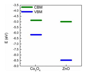
Fig. 6 Band alignment between ZnO and Co<sub>3</sub>O<sub>4</sub> calculated using the GW0 method. The zero of the energy corresponds to the vacuum energy.
