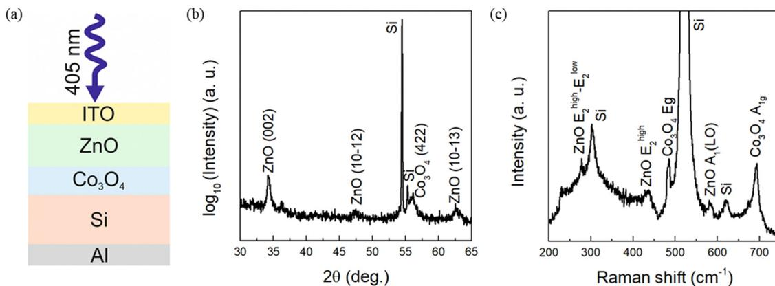
Fig. 1 Structural characterization of the Si/Co<sub>3</sub>O<sub>4</sub>/ZnO heterojunction. (a) Illustration of the device cross section. (b) XRD pattern and (c) Raman spectrum.
