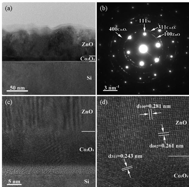
Fig. 2 (a) TEM image at low magnification of the Si/Co<sub>3</sub>O<sub>4</sub>/ZnO structure, (b) corresponding SAED pattern of the TEM image with four peaks indexed, (c) HRTEM image of the analyzed sample showing the interface between Si/Co<sub>3</sub>O<sub>4</sub> and Co<sub>3</sub>O<sub>4</sub>/ZnO, (d) magnified view of the Co<sub>3</sub>O<sub>4</sub>/ZnO interface with both layers oriented relatively to the electron beam.
