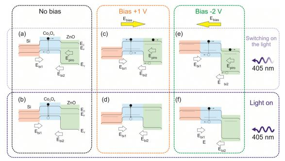
Fig. 7 Band diagram schemes of the Si/Co<sub>3</sub>O<sub>4</sub>/ZnO structure for different conditions. (a), (c) and (e) while the light is being turned on for different bias conditions; (b), (d) and (f) with light on for different bias conditions
