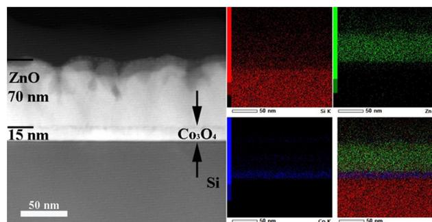
Fig. 3 High-angle annular dark-field scanning transmission electron microscopy (HAADF-STEM) image of Si/Co<sub>3</sub>O<sub>4</sub>/ZnO structure and energy dispersive X-ray spectroscopy elemental mapping performed on the HAADF-STEM image showing the spatial distribution of Zn, Co and Si elements across the analyzed STEM image. The combined color map was obtained by overlapping the Si, Co and Zn maps.
