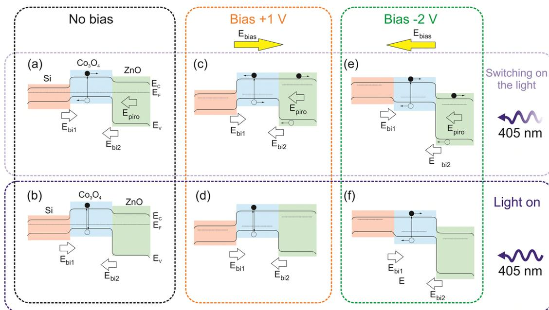
Fig. 7 Band diagram schemes of the Si/ $\text{Co}_3\text{O}_4$ /ZnO structure for different conditions. (a), (c) and (e) while the light is being turned on for different bias conditions; (b), (d) and (f) with light on for different bias conditions.
