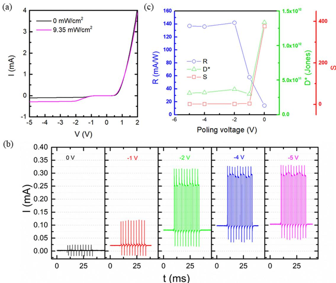
Fig. 5 (a) *I-V* curves for the Al/Si/Co<sub>3</sub>O<sub>4</sub>/ZnO/ITO device in the dark and under illumination with a power density 9.35 mW cm<sup>-2</sup>. (b) *I-t* curves for the Al/Si/Co<sub>3</sub>O<sub>4</sub>/ZnO/ITO without and with external bias. (c) Variation of responsivity, detectivity and sensitivity as a function of external bias.
