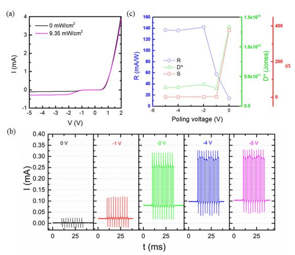
Fig. 5 (a) I-V curves for the Al/Si/Co<sub>x</sub>O<sub>4</sub>/ZnO/ITO device in the dark and under illumination with a power density 9.35 mW cm<sup>-2</sup>. (b) I-t curves for the Al/Si/Co<sub>3</sub>O<sub>4</sub>/ZnO/ITO without and with external bias. (c) Variation of responsivity, detectivity and sensitivity as a function of external bias.
