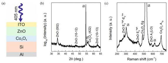
Fig. 1 Structural characterization of the Si/Co<sub>3</sub>O<sub>4</sub>/ZnO heterojunction. (a) Illustration of the device cross section. (b) XRD pattern and (c) Raman spectrum
