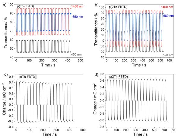
Fig. 12 Kinetic curves recorded during electrochromic switching of polymer films between the neutral and first oxidized states: (a) transmittance of p(Th-FBTD); (b) transmittance of p(2Th-FBTD); (c) chronocoulometry plot for p(Th-FBTD); (d) chronocoulometry plot for p(2Th-FBTD)
