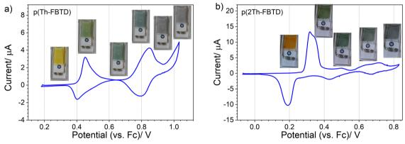
Fig. 11 Cyclic voltammograms of polymer films on ITO electrodes in 0.1 M Bu<sub>4</sub>NPF<sub>6</sub>/DCM as the supporting electrolyte solution: (a) p(Th-FBTD); (b) p(2Th-FBTD). Insets: Photographs of polymer films at the given potential. Scan rate 2 mV s<sup>-1</sup>.
