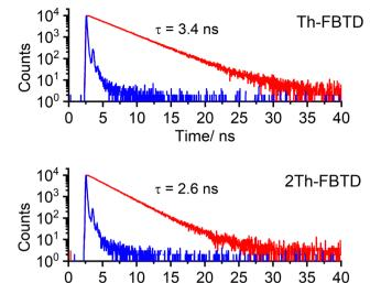
Fig. 4 Photoluminescence decay of Th-FBTD and 2Th-FBTD in a degassed dilute ( $c = 10^{-6}$  M) toluene solution: TCSPC decay traces with collection at  $\lambda_{PL}$  = 550 nm (red lines); instrument response function, IRF (blue lines)
