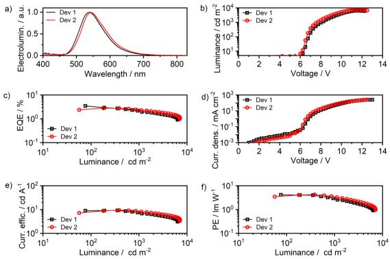
Fig. 6 Characteristics of OLED devices 1 (using **Th-FBTD** as an emitter) and 2 (using **2Th-FBTD** as an emitter): (a) electroluminescence spectra at 10 V; (b) luminance vs. voltage; (c) external quantum efficiency (EQE) vs. luminance; (d) current density vs. voltage; (e) current efficiency vs. luminance; (f) power efficiency (PE) vs. luminance.
