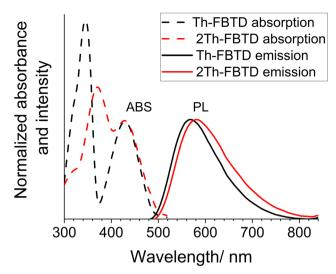
Fig. 3 UV-Vis absorption spectra (dashed lines) and normalized photoluminescence spectra (continuous lines) of investigated benzothiadiazole derivatives **Th-FBTD** and **2Th-FBTD** in  $c = 10^{-6}$  M DCM solution. The spectra are normalized to the lowest absorption band of each respective molecule
