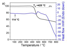
Fig. 1  $\,$  TGA and DSC curves for (a) Th-FBTD and (b) 2Th-FBTD.
