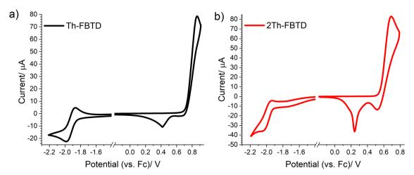
Fig. 5 Cyclic voltammograms recorded for 1.0 mM solution of (a) Th-FBTD and (b) 2Th-FBTD in 0.1 M Bu<sub>4</sub>NPF<sub>6</sub>/DCM electrolyte. Scan rate 0.1 V s<sup>-1</sup>.
