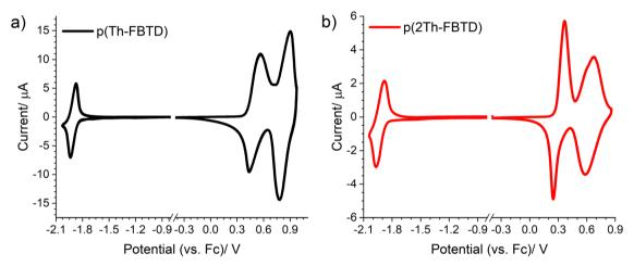
Fig. 8 Cyclic voltammograms of the electrodeposited layers of (a) **p(Th-FBTD)** and (b) **p(2Th-FBTD)**, in a monomer-free 0.1 M  $Bu_4NPF_6/DCM$  electrolyte solution. Scan rate 0.1 V  $s^{-1}$ .
