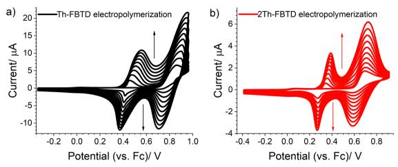
Fig. 7 Potentiodynamic electropolymerization of (a) **Th-FBTD** and (b) **2Th-FBTD** (0.5 mM solutions), using a platinum working electrode immersed in 0.1 M Bu<sub>4</sub>NPF<sub>6</sub>/DCM electrolyte (10 cycles). Scan rate 0.1 V s<sup>-1</sup>. The arrows indicate the direction of the current increase in the voltammograms.
