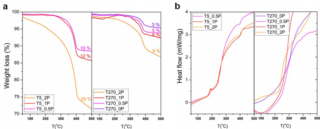
Fig. 5 (a) Thermogravimetric analysis of the synthesized samples of  $\text{Bi}_{19}\text{S}_{27}\text{I}_3$  at different reaction times and PEG:Bi molar ratios. (b) Differential scanning calorimetry of the synthesized samples of  $\text{Bi}_{19}\text{S}_{27}\text{I}_3$  at different reaction times and PEG:Bi molar ratios.
