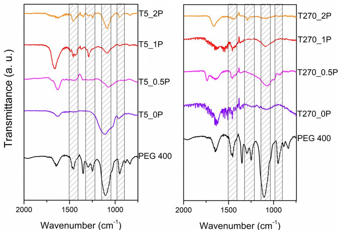
Fig. 4 FTIR spectra of the Bi<sub>19</sub>S<sub>27</sub>I<sub>3</sub> samples compared with PEG 400 for 5 and 270 minutes of reaction. The bands of interest are marked in both graphs.
