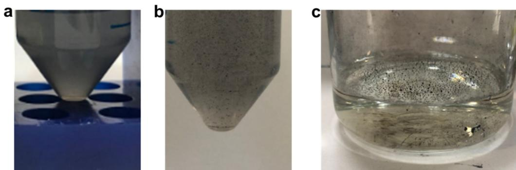
Fig. 8 (a) Sample T270\_1P suspended in Cr(vi) aqueous solution in a falcon tube; (b) sample T270\_0P suspended in Cr(vi) aqueous solution in a falcon tube; (c) sample T270\_0P in Cr(vi) aqueous solution in the photocatalysis reactor.
