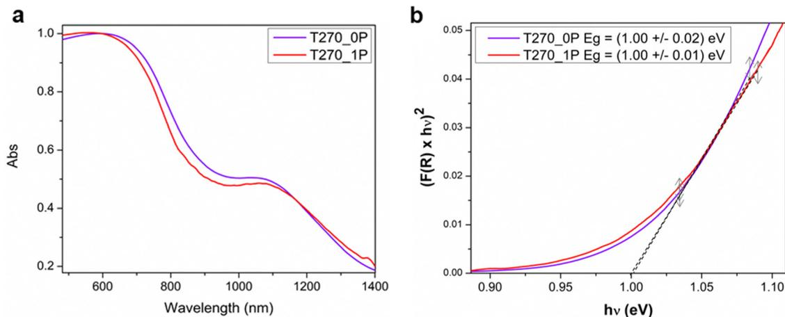
Fig. 6 (a) UV-vis absorption spectra of the T270\_0P and T270\_1P samples. (b) Tauc plot after Kubelka–Munk transformation for the direct band gap of  $\text{Bi}_{19}\text{S}_{27}\text{I}_3$  in samples T270\_0P and T270\_1P. Calculated values are shown with the error of fitting.
