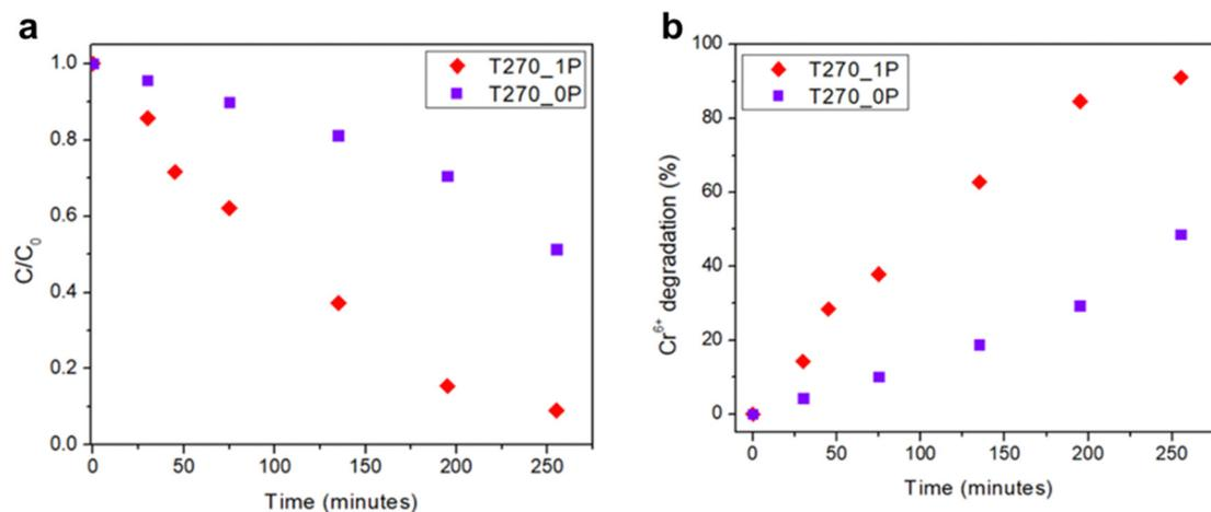
Fig. 7 (a)  $\text{Cr}(\text{vi})$  reduction using  $\text{Bi}_{19}\text{S}_{27}\text{I}_3$  synthesized with and without PEG as the capping agent as photocatalysts, and (b) variation in the % of  $\text{Cr}(\text{vi})$  reduction over time.
