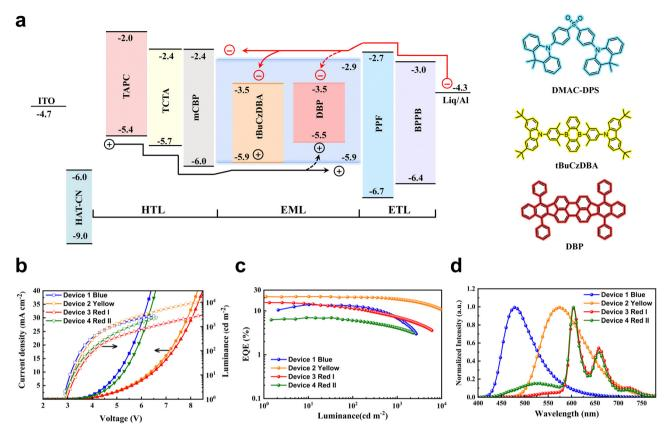
Fig. 1 (a) Energy diagram and molecular structures of emitters adopted in monochrome blue/yellow/red OLEDs. (b) Current density-voltageluminance (J-V-L) curves of monochrome OLEDs. (c) EQE-luminance characteristics of monochrome blue/yellow/red OLEDs. (d) EL spectra of monochrome blue/yellow/red OLEDs at 100 cd m<sup>-2</sup>
