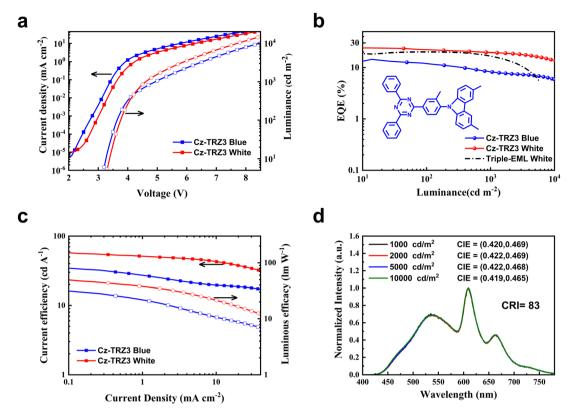
Fig. 4 (a) Current density-voltage-luminance curves of blue and white devices based on Cz-TRZ3; (b) EQE-luminance characteristics of blue and white devices based on Cz-TRZ3. The black dashed line is a triple-EML WOLED based on DMAC-DPS (W3). The insert is the molecular structure of Cz-TRZ3; (c) current efficiency and luminous efficacy versus current density curves of blue and white OLED based Cz-TRZ3; (d) EL spectra of white devices based on Cz-TRZ3 under different luminance.
